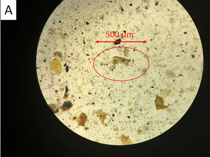
Figure S4C: polarised light study of a thin C 2 N 2D flake (circles). A): normal light (red circle, 300); B): the same flake under cross polarized light and C) same sample upon rotation (yellow circles/arrows on B) and C) as a guide to the eye). The appearance of the flake alternatively goes brighter and darker as a function of the angle.
