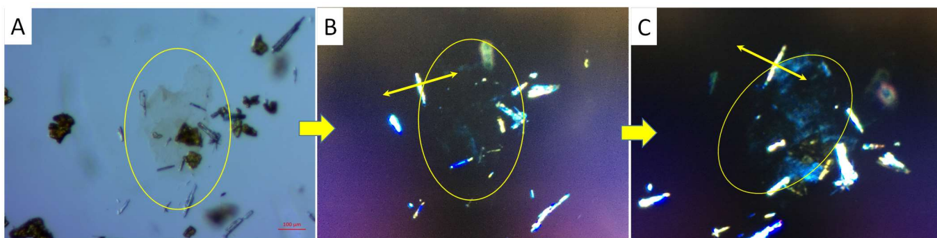
Figure 22: polarised light study of a thin CTF 2D flake (yellow circle). A): normal light; B): the same flake under cross polarized light and C) same sample upon rotation (yellow arrows on B and C as a guide to the eye). The appearance of the flake alternatively goes brighter and darker as a function of the angle. Bright crystals of the starting product are also observed.
