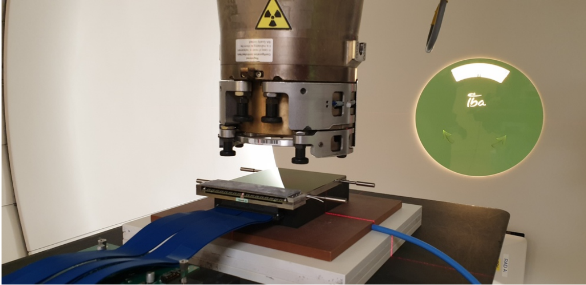
Figure 3. Photograph of the vM2428 detector during setup, positioned 7 cm from the surface of the collimator.
