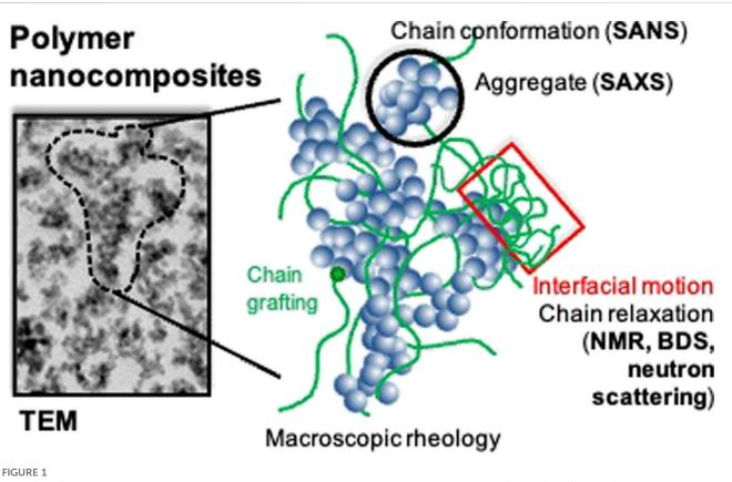
Illustration of a polymer nanocomposite with a spectrum of techniques used to characterize the structure and dynamics of nanoparticles and polymer, with a particular focus on the interfacial (possibly grafted) polymer layer.
