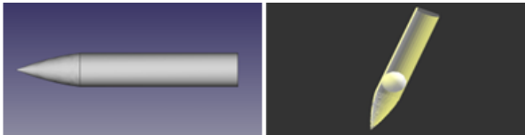
Fig. 6 Projectile design: 3D modeling in YADE
