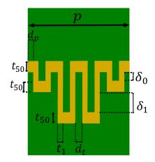
Figure 1. Geometry of the proposed unit cell.
