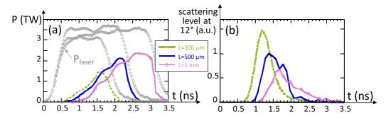
FIG. 5. (a) Laser pulse and power transmitted in the original beam aperture for shots in 7 mg/cc foams with lengths 300  $\mu$ m, 500  $\mu$ m, and 1 mm. (b) Corresponding power scattered at  $\theta_s = 12^\circ$ .
