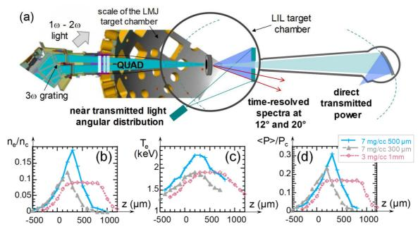
FIG. 1. (a) Sketch of the experimental setup. (b) Electron density and (c) temperature profiles computed at  $t \sim 1.35$  ns for three different foams; the foam entrance plan is in z = 0; (d) corresponding  $\langle P \rangle / P_c$ , where  $\langle P \rangle$  is the power computed in a speckle at  $1.5 \times 10^{15}$  W/cm<sup>2</sup>.
