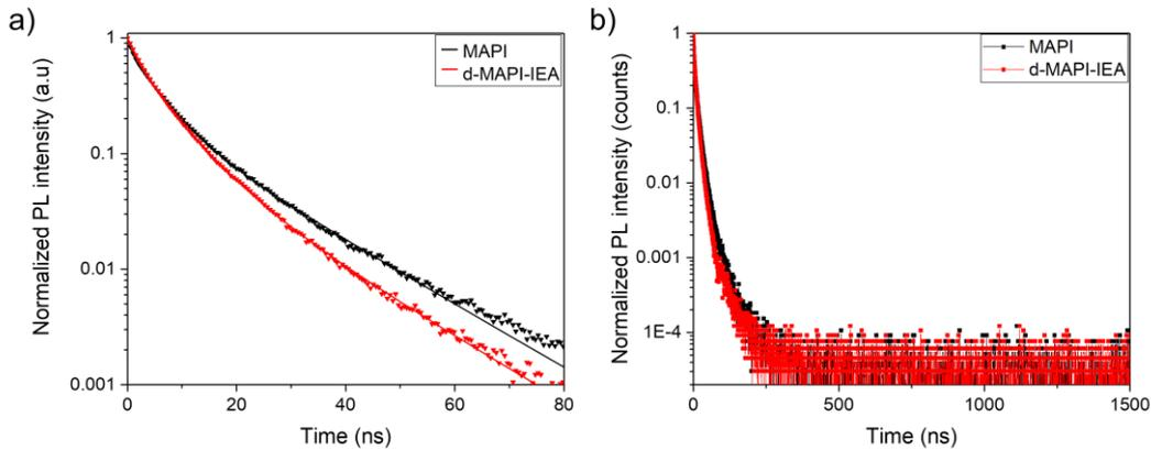
Figure 6: Normalized time-resolved photoluminescence of MAPbI<sub>3</sub> and d-MAPI-IEA films on FTO/c-TiO<sub>2</sub>/m-TiO<sub>2</sub> substrates. (a) Zoom between 0-80 ns. (b) Measurement over 1500 ns. The full lines are the fitting curves obtained from the triple exponential fitting of the experimental points (downward triangles).
