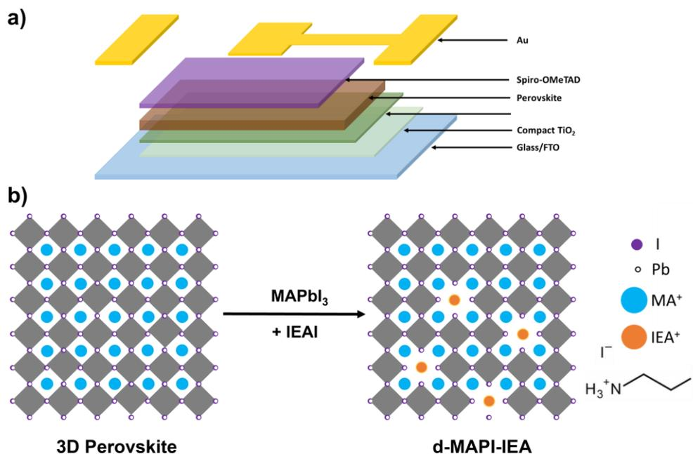
Figure 1: (a) Exploded schematic view of the perovskite solar cell structure. (b) Schematic representation of classic 3D MAPbI<sub>3</sub> and of 3D d-MAPI-IEA perovskite formed after partial substitution of PbI<sup>+</sup> units by IEA<sup>+</sup> cations.
