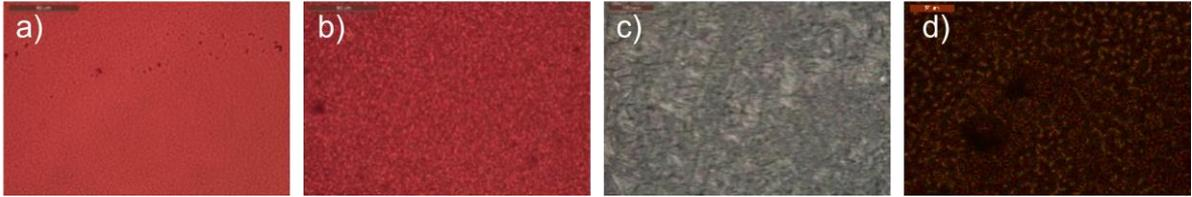
Figure 5: Optical microscope pictures of d-MAPI-IEA films for Pb/MA/IEA molar ratios of (a) 1/0.5/1 (b) 1/0.66/0.66 (c) 1/0.75/0.5 and (d) 1/0.8/0.4 (IEA<sup>+</sup> content decreases from a) to d))
