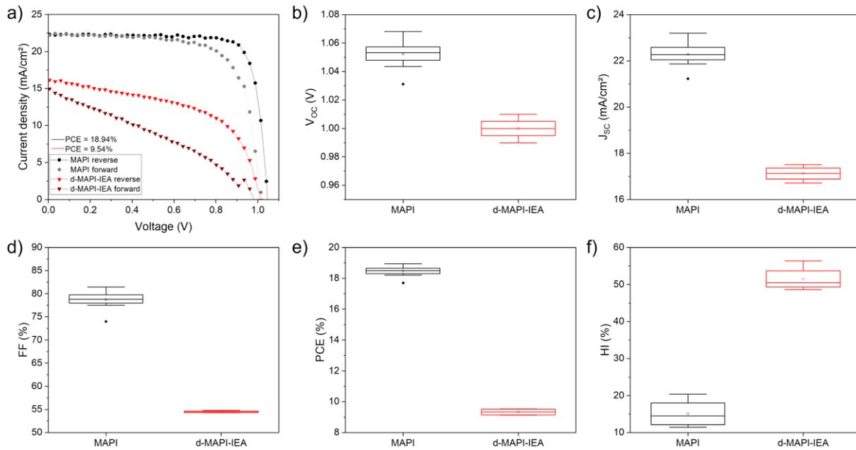
Figure 7: (a)  $J$ - $V$  curves of best MAPbI<sub>3</sub> and d-MAPI-IEA devices with measured reverse scan PCEs. (b-f) Box charts of MAPbI<sub>3</sub> and d-MAPI-IEA PSCs  $J$ - $V$  parameters,  $PCE$  and  $HI$ .
