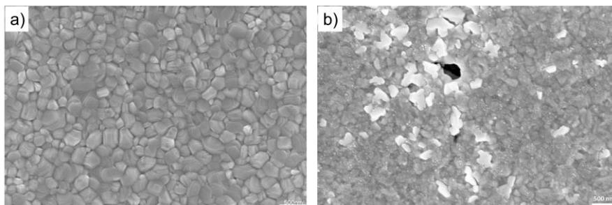
Figure 3: Top-view SEM of (a) MAPbI<sub>3</sub> and (b) d-MAPI-IEA perovskite films. Scale bar: 500 nm.
