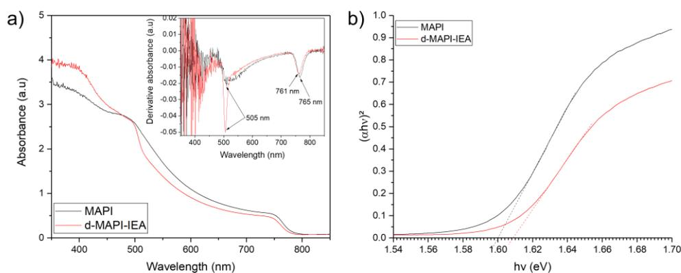
Figure 4: (a) UV-Visible spectra of MAPbI<sub>3</sub> and d-MAPI-IEA perovskite films. Inset: the associated derivative absorbance. (b) Tauc Plot associated to the UV-Visible absorbance spectra.
