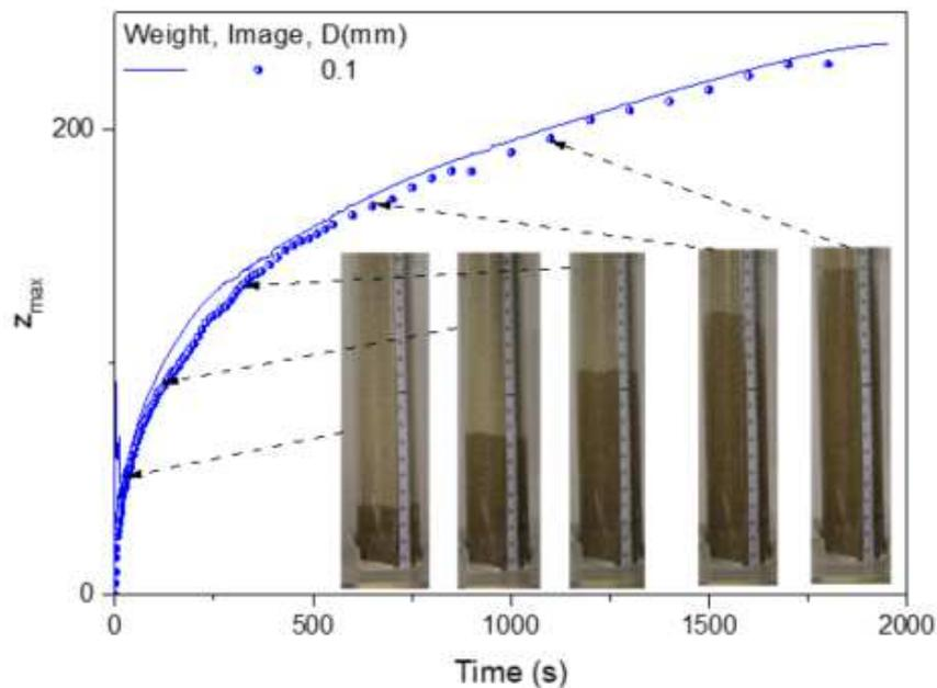
Figure 9. The liquid height rises for homogeneous domain, using the image processing (the discrete dots), and weighting techniques (the continuous line). The inserted chosen images are at the time points of 70s (5cm), 140s (9.5cm), 280s (13cm), 560s (16.5cm) and 1120s(19cm), respectively
