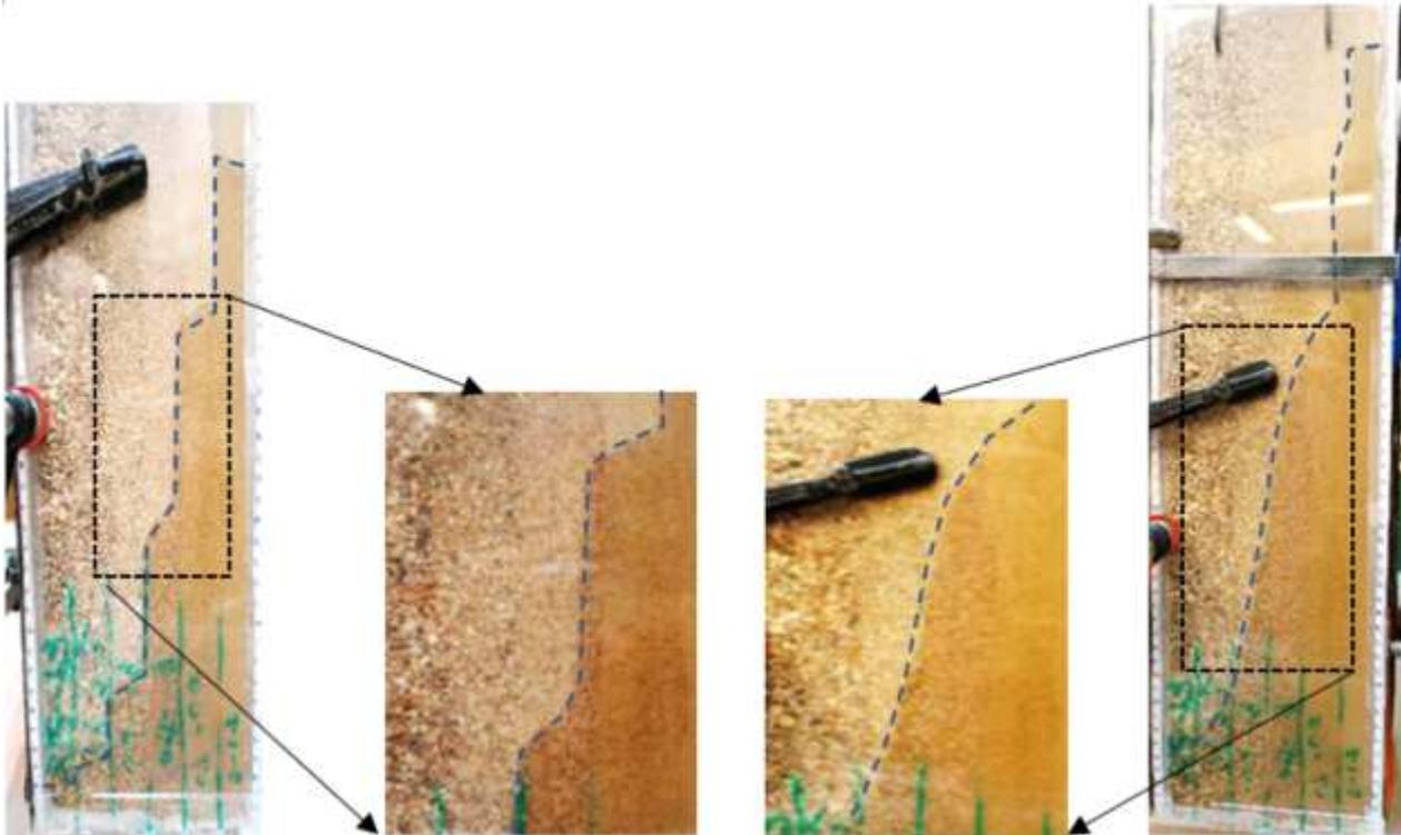
Figure 15. Liquid rise interface shape at two different time points (early – left and later – right), and their corresponding zooms (in central position)
