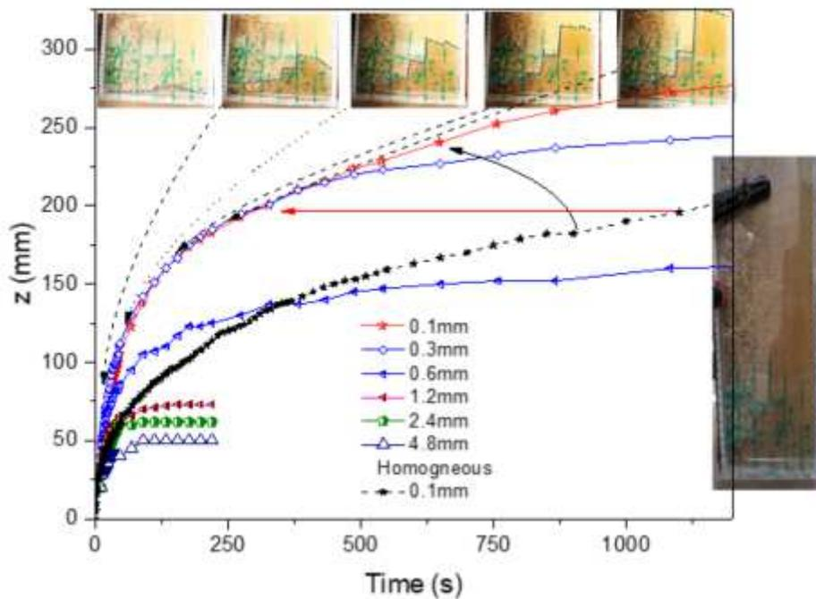
Figure 14. Liquid height rises for heterogeneous multilayer domain and the corresponding reference of homogeneous 0.1 mm case, images inserts illustrate the top shape of the liquid rise over such heterogenous domain.
