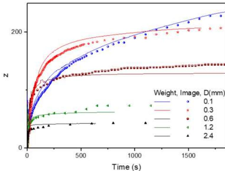
Figure 10. The height liquid rises versus time for different homogeneous domain, using both the image processing (dots) and weighting technique (lines)
