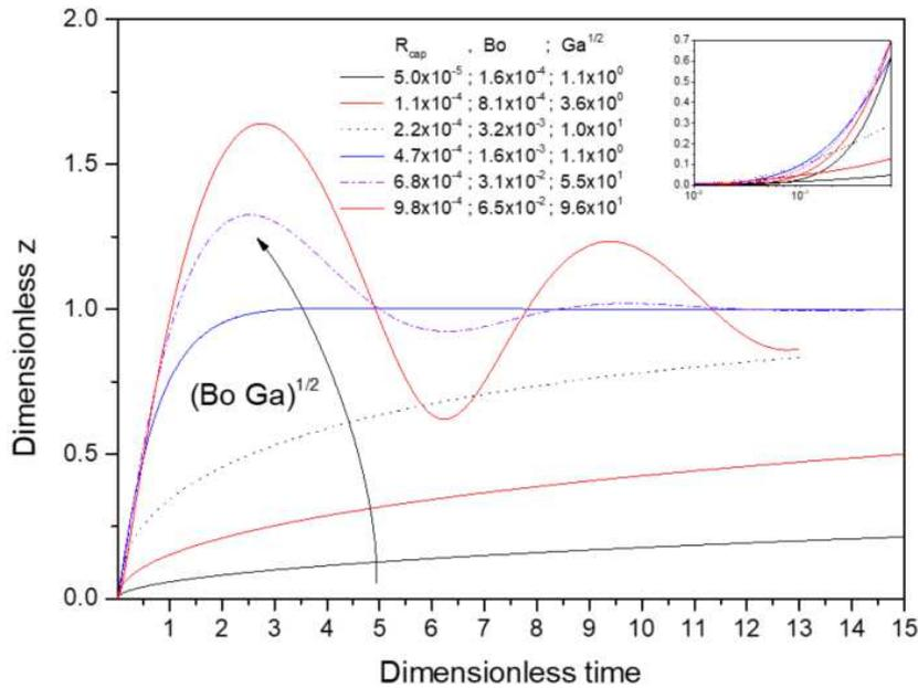
Figure 3. The capillary rise over time for different  $\Omega$
