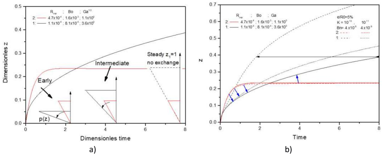
Figure 6. Liquid height versus time for two adjacent layers of different equivalent radius, without horizontal exchange (impermeable on the interface) a) and with exchange (permeable) b)
