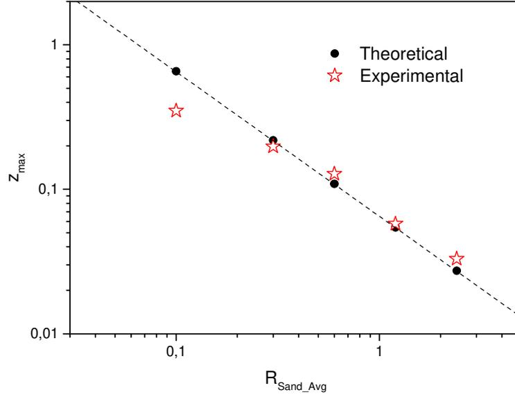
Figure 11. The effect of sand equivalent radius on the maximum liquid height rise (homogeneous domain)
