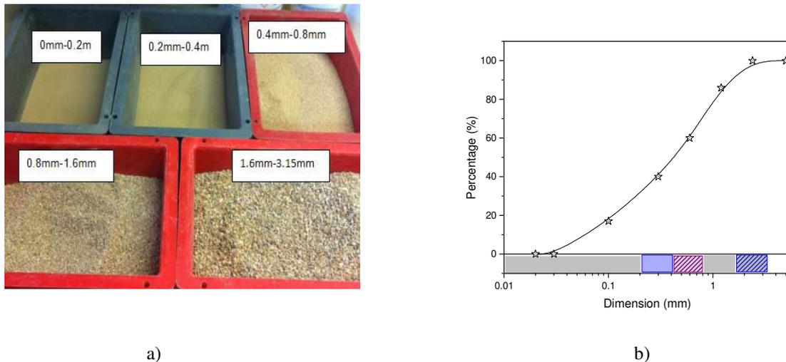
Figure 7. Sands of different sizes after filtering a), Integral percentage of particle size curve b)
