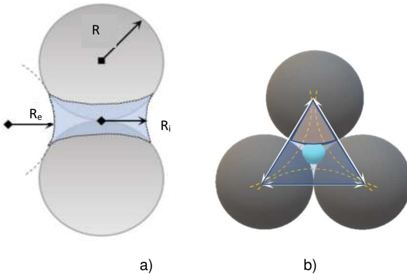
Figure 4. Liquid bridge and radii of curvature a) and the equivalent capillary radius [36]
