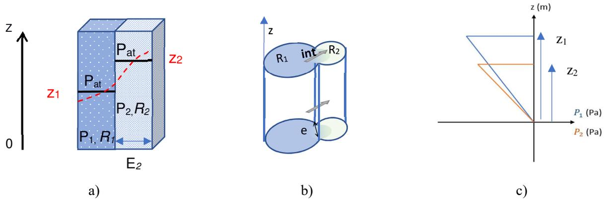
Figure 5. Two layers of liquid exchange a), equivalent capillary case b), and the pressure on the two capillaries in vertical direction c)
