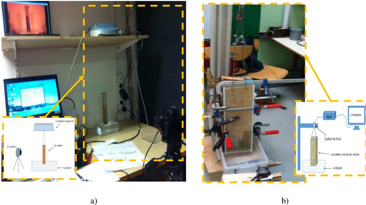
Figure 8. Experimental devices for homogenous sands imbibition a) and heterogeneous with multi layers b), using balance or force sensor for mass recording and camera or capillary height monitoring
