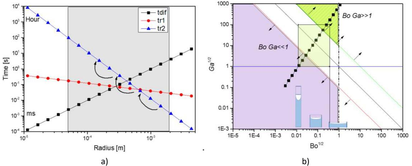
Figure 2. The three involved characteristic times a), different regimes summarized by the two dimensionless numbers ( $Bo$  ;  $Ga$ ) b).
