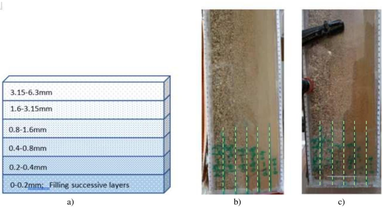
Figure. 13: Heterogeneous domain of six layers with sand diameters of 0.1 mm, 0.3 mm, 0.6 mm, 1.2 mm, 2.4 mm and 4.8 mm a), the vertical domain before imbibition b) and after imbibition c)
