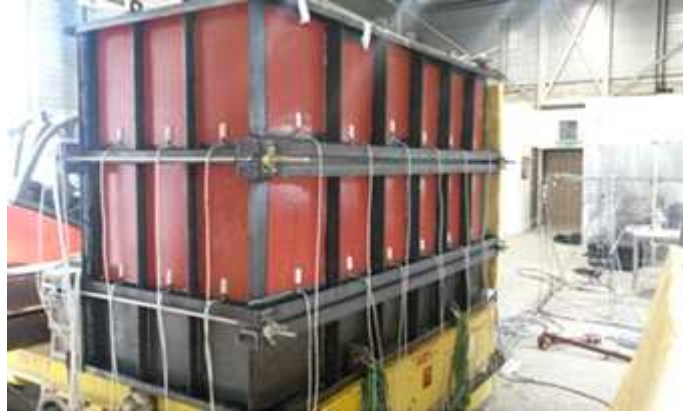
Figure 6 : DEF mock-up's early-age temperature regulation system
