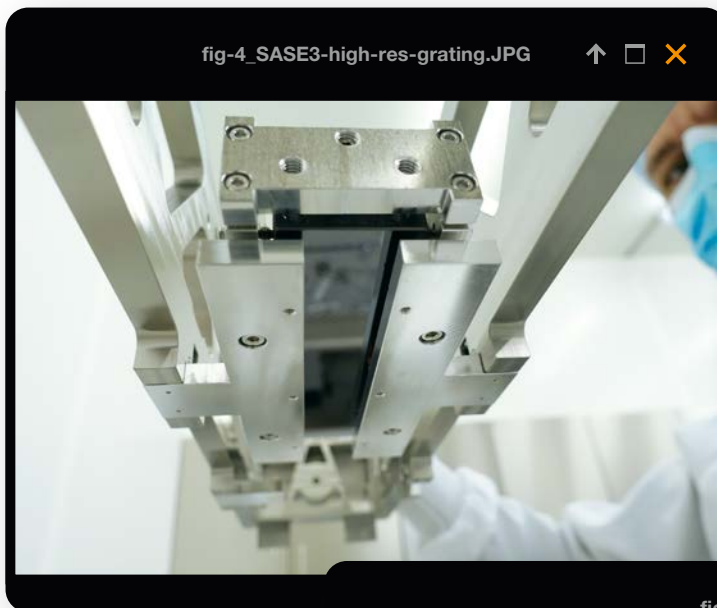
Figure 4: Photograph taken upwards looking at the face of the new high-resolution grating for the SASE3 soft X-ray monochromator, installed on the mirror mount in the metrology laboratory
