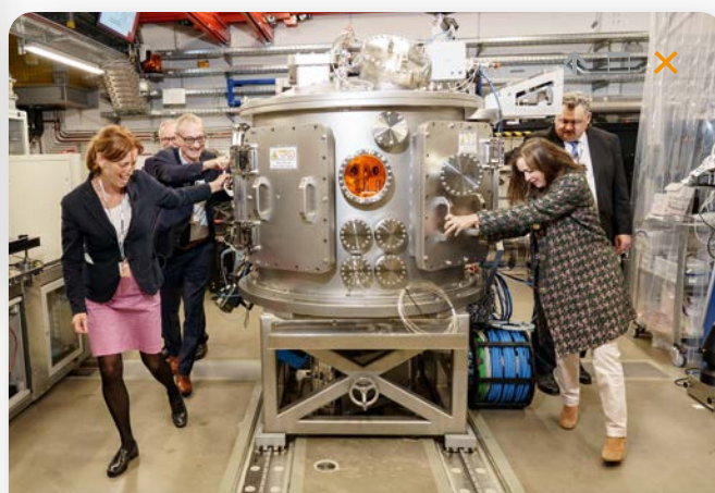
The HiBEF interaction chamber is being pushed into the beam.
