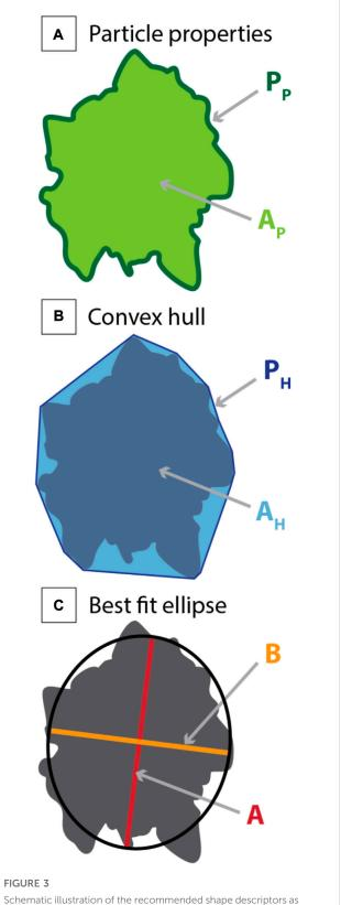
Schematic illustration of the recommended shape descriptors as defined by Liu et al. (2015). (A) Key pyroclast properties consisting of the pyroclast perimeter,  $P_P$  and the pyroclast area,  $A_p$ . (B) The area,  $A_H$  and perimeter,  $P_H$  of the bounding convex hull. (C) The major,  $A_H$  and the minor,  $A_H$  axes of the best fit ellipse.
