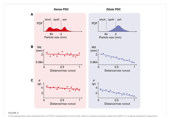
(right). (A) shows conceptual grain size distributions, (B) an illustration of the change in median (Md) and (C) sorting coefficient (φ) within a flow with distance from source.
