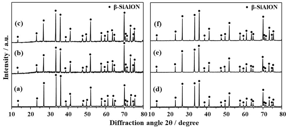
**FIGURE 1** XRD patterns of polymer-derived  $\beta$ -SiAlON:  $\text{Eu}^{2+}$  phosphor samples: (a) **1800°C-NHA63E1** [20], (b) **1800°C-NHA66E1**, (c) **1800°C-NHA69E1** samples and reference samples of (d) **PMM63-1h**, (e) **PMM63-8h** and (f) **PMM-8h**
