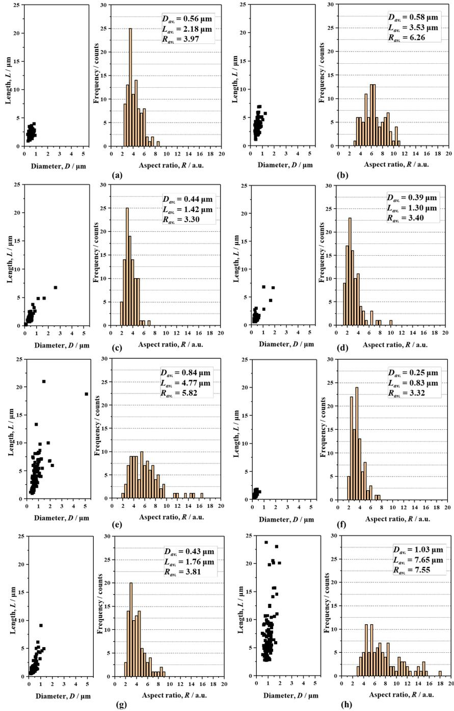
**FIGURE S2** Grain size distribution and average grain diameter, length and aspect ratio evaluated for the selected samples of (a) 1800°C-NA90E1 [19] (b) 1800°C-NA90E5 [19], (c) 1800°C-NA63E1 [20], (d) 1800°C-NHA63E1 [20], (e) 1800°C-NHA66E1 and reference samples of (f) PMM63-1h, (g) PMM63-8h and (h) PMM-8h
