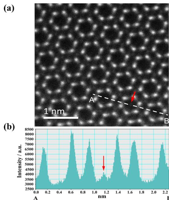
**FIGURE 6** (a) HAADF-STEM image of **1800°C-NA63E1** sample [20] showing (a) typical six-membered rings of  $\beta\text{-SiAlON}$  and (b) the Z contrast profile along with the A-B line across the atomic channel shown in (a).
