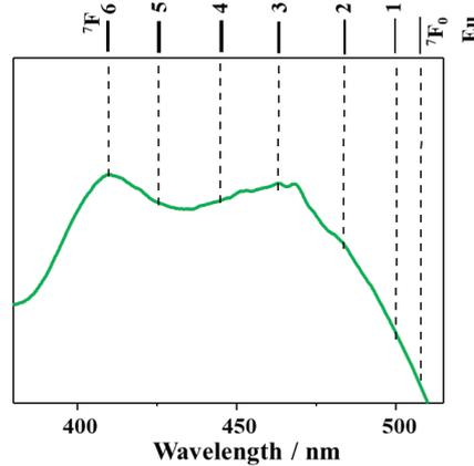
**FIGURE 5** Amplified excitation spectrum of the **1800°C-NA63E1** sample [20] with the <sup>7</sup>F<sub>J</sub> (J=1-6) energy levels of Eu<sup>3+</sup> cation
