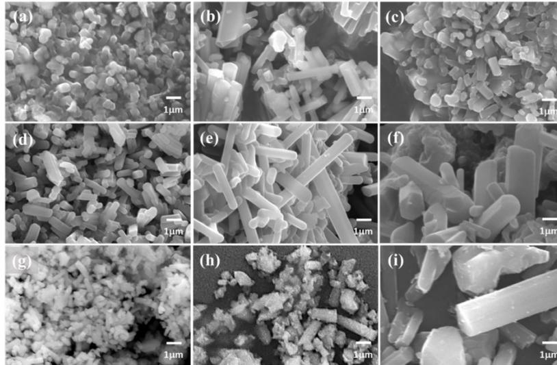
**FIGURE 2** SEM images showing morphology of polymer-derived  $\beta$ -SiAlON:  $\text{Eu}^{2+}$  phosphor samples: (a) 1800°C-NA90E1 [19], (b) 1800°C-NA90E5 [19], (c) 1800°C-NA63E1 [20], (d) 1800°C-NHA63E1 [20], (e) 1800°C-NHA66E1, (f) 1800°C-NHA69E1 and reference samples fabricated through the conventional powder metallurgy route: (g) PMM63-1h, (h) PMM63-8h and (i) PMM-8h
