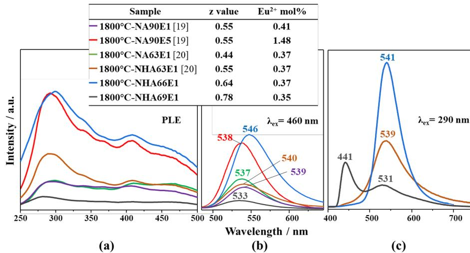
**FIGURE 4** PL properties of **1800°C-NHA66E1** and **1800°C-NHA69E1** samples along with **1800°C-NA90E1** [19], **1800°C-NA90E5** [19], **1800°C-NA63E1** [20] and **1800°C-NHA63E1** [20] samples. (a) Excitation spectra monitored at appropriate maximum emission wavelengths shown in (b), and emission spectra under excitation at (b) 460 nm, and (c) 290 nm
