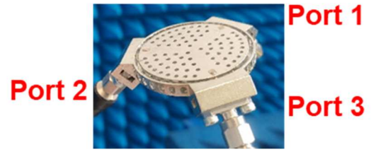
Fig. 6. Prototype 1: 3-port antenna prototype with direct SMA connectors excitations.
