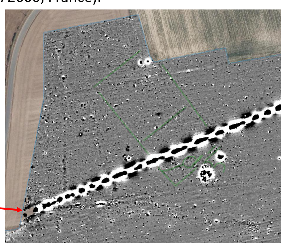
Example of drainage ditches Magnetic map of the Roman site of Roullée (72600, France).
