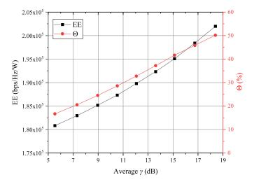
Fig. 7. EE and  $\Theta$  of the aggregated network versus average  $\gamma$  for settings  $\alpha=\beta=0.5$  and  $R^{\rm thr}=10$  bps/Hz.
