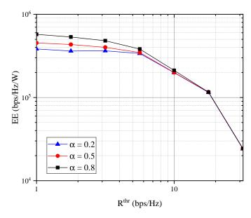
Fig. 3. EE of the aggregated network versus  $R^{\rm thr}$  for different  $\alpha$  values.
