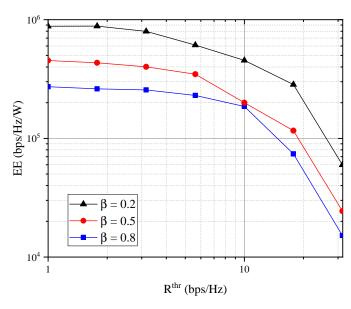
Fig. 4. EE of the aggregated network versus  $R^{\mathrm{thr}}$  for different  $\beta$  values.
