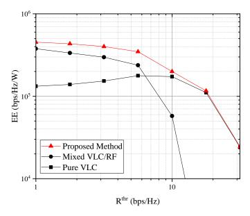
Fig. 2. EE versus  $R^{\rm thr}$  comparison between non-aggregated special cases and aggregated approach for  $\alpha=\beta=0.5$ .
