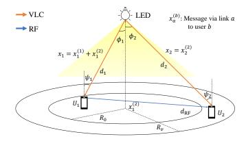
Fig. 1. System model to implement the proposed cooperative VLC NOMA protocol. Cell-center user  $(U_1)$  performs SIC to recover its own message and the message to be forwarded over the RF sidelink. Cell-edge user  $(U_2)$  aggregates the data rate from its own VLC reception (no SIC) and the sidelink communication.
