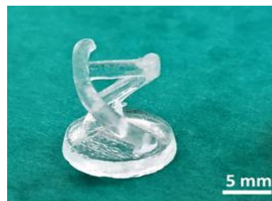
Figure 25. Silica part after de-binding and sintering [91].
