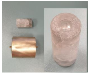
Figure 8. Thermally cured part in a conductive sleeve. All the material accessible to the exothermic reaction is transformed into the polymer (see photograph on the right).
