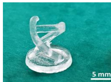
Figure 25. Silica part after de-binding and sintering [91].
