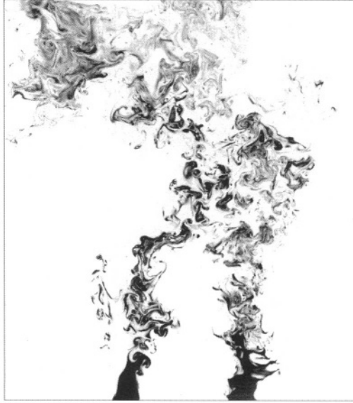
Figure 7 Two nearby sources discharging in a turbulent medium in which they mix.
