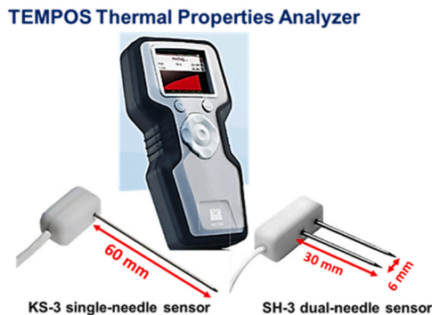
Fig. 5. The TEMPOS thermal properties analyzer with KS-3 and SH-3 sensors.
