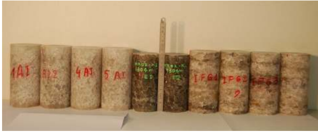
Fig. 7 Ten samples set in the gallery at the beginning of the test (IFG#1 sample is called Gorleben #1, or Go#1 in this paper)
