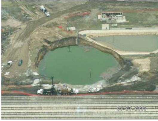
Fig. 11. Well # 19 sinkhole view and vertical cross-section, after. 21 A deviated well and a sonar survey proved that sediments flowed into the cavern through a narrow central hole.
