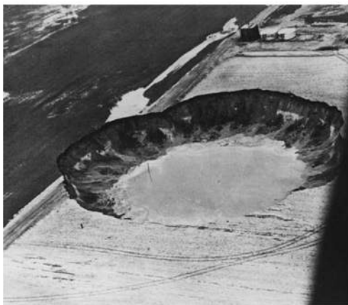
Fig. 12. Panning Sinkhole, Kansas, left [Photo taken on April 24, 1959, by Larry Panning 21 ] and tentative explanation of the final collapse, after 21 : water pressure and water level dropped in the cavern after plugging severed the hydraulic connection between the cavern and the shallow aquifer, leading to final collapse.
