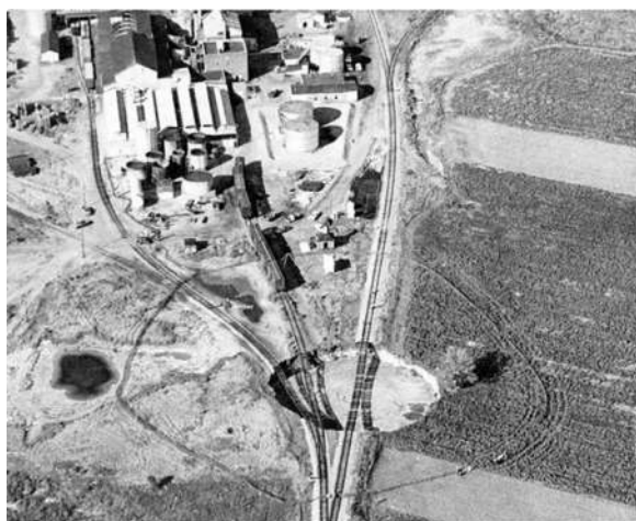
Fig. 10. Cargill salt plant, Hutchinson, Kansas, 1974. 21 (Some 14 h after the collapse, the sinkhole diameter was 200 ft.) (Photograph by Hutchinson News, October 21, 1974.).
