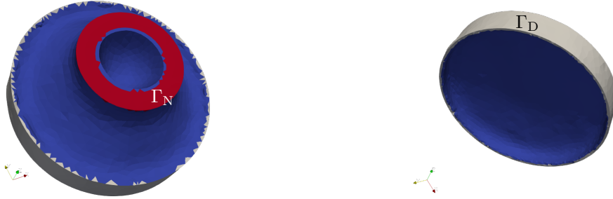
FIG. 7. Structure of the 3D disc structure. The region \Gamma_N where the random load is applied is marked in red, while the clamping region \Gamma_D is highlighted in gray.
