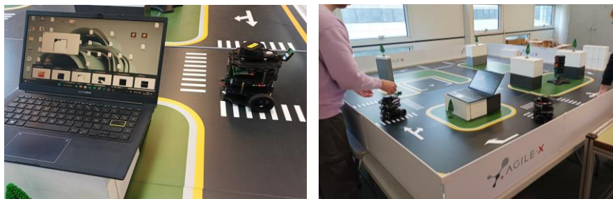
Figure 5: In situ validation and tests of system behavior. The robot must perform autonomous navigation task in hard lighting conditions making IA model road recognition complex problem requiring a deep neural network challenging computing resources as well as system robustness.
