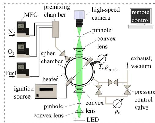
Fig. 2. Schematic of the microgravity experimental setup.
