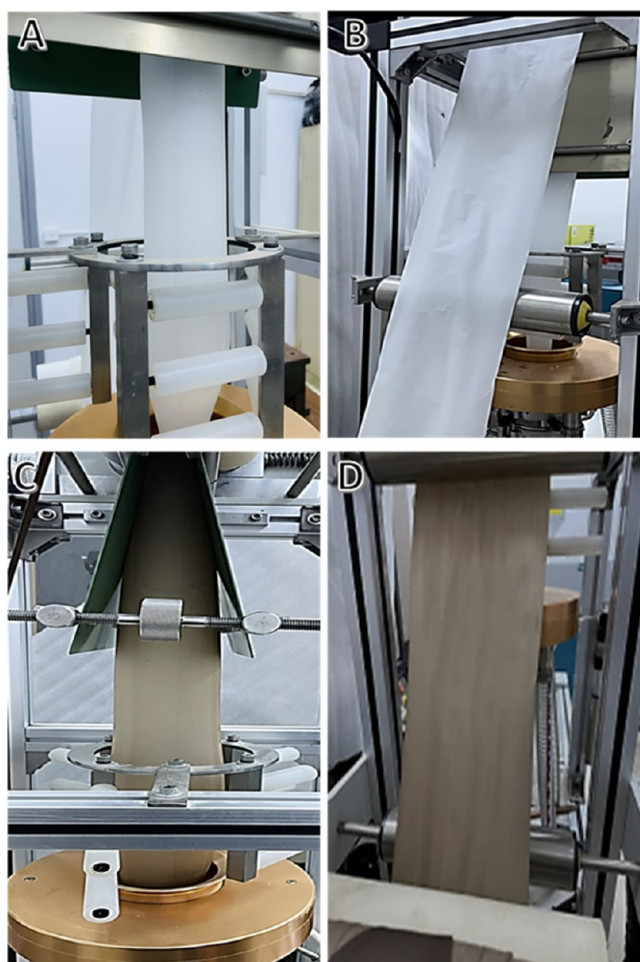
Figure 10. Photos showing the production of thin film by blown-film extrusion from PBAT/TPS 60/40 blends without LCNFs (A, B) and with 8 wt % LCNFs (C, D).
