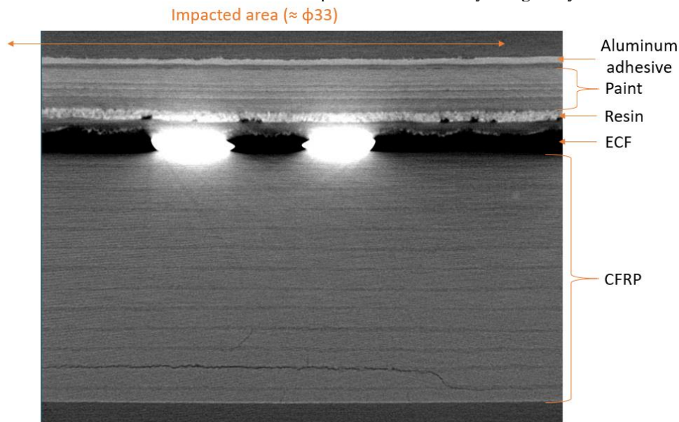
Figure 7 Microtomography cross section view of a post-mortem CCR+ECF+Paint sample submitted to a laser shot with a 1-centimeter thick glass confinement and a flux of approximately- 4.68 GW.cm -2 . Voxel size of 39.3 µm 3 .
