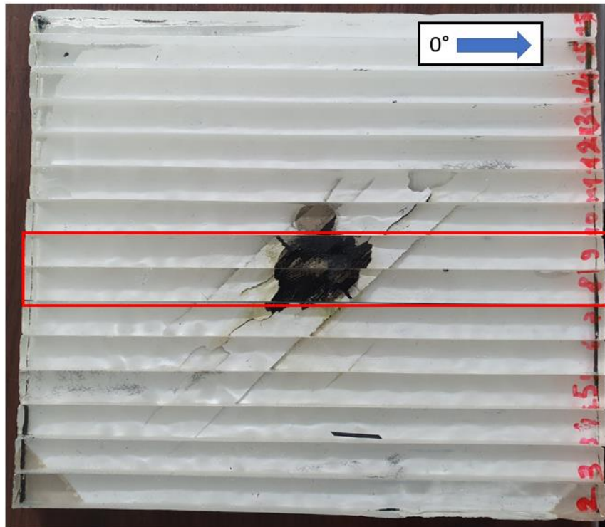
Figure 10 Post-mortem lightning strike CFRP+ECF+Paint sample coated in resin and cut for the microscopic analysis. Slices 8 and 9 framed in red.
