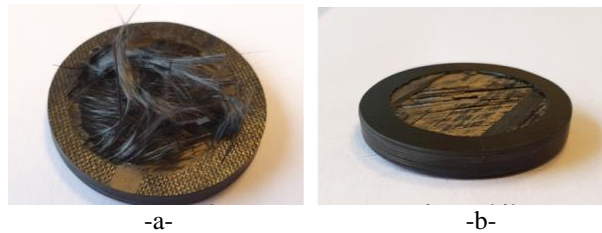
Figure 3 Typical damage produced by electron beam on 35 mm diameter CFRP laminate. -a-: Front face, explosion. -b-: Back face spalling.
