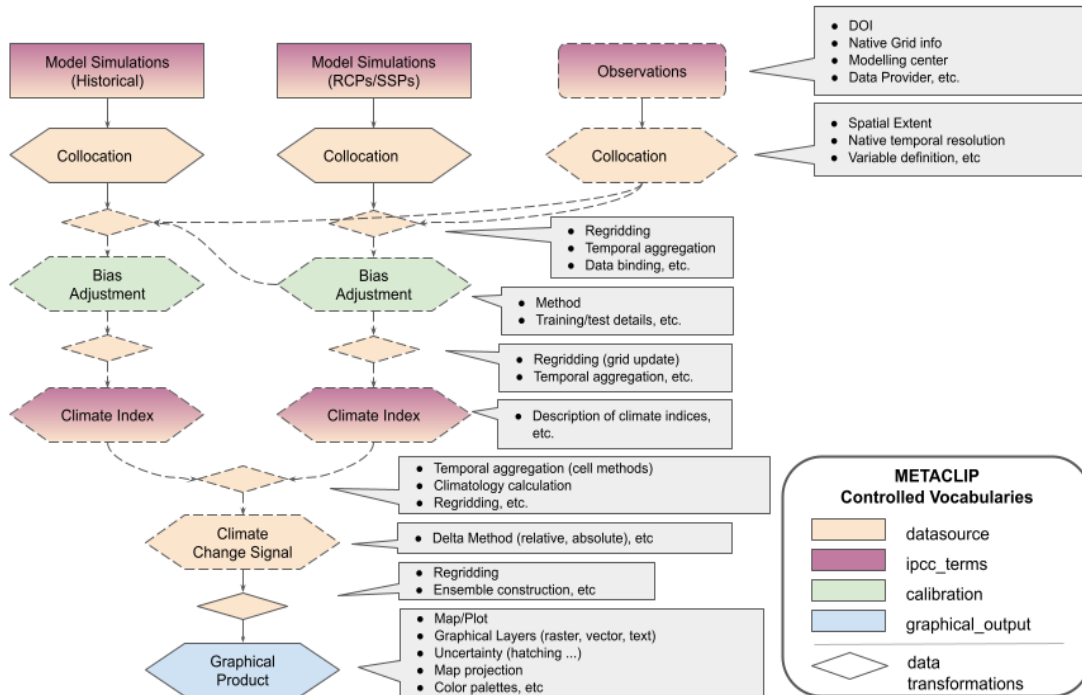
Fig 2. Schematic representation of an Atlas product generation workflow (a Bias adjusted Climate index Delta change similar to the map displayed in Fig. 3). The main steps involve database description, subsetting and data transformation, and finally graphical product generation. META CLIP specifically considers the different intermediate steps consisting of various data transformations, statistical adjustment, climate index calculation and graphical product generation, providing a semantic description of each stage and the different elements involved. The different controlled vocabularies describing each stage are indicated by the colors. The gradient indicates that both ipcc_terms and datasource vocabularies are involved, usually meaning that specific individual instances have been defined in ipcc_terms extending generic classes of the datasource vocabulary (Table 1).
