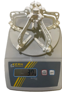
Fig. 7: Weight of the scaled gripper for the quadrotor used
