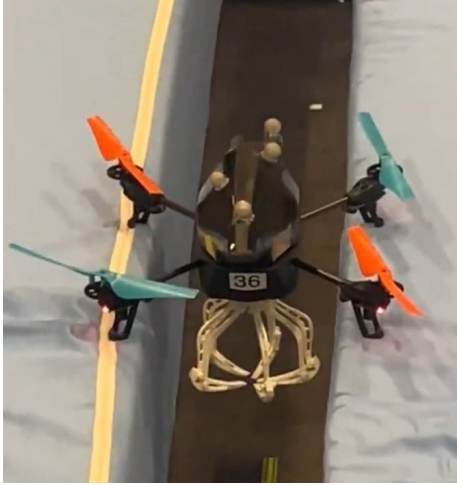
Fig. 9: Drone Parrot A.R. Drone 2.0 with the designed gripper mounted
