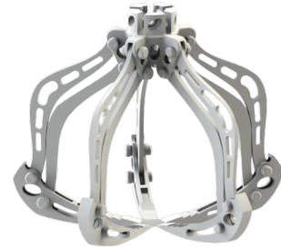
Fig. 3: Gripper in closed position while flying
