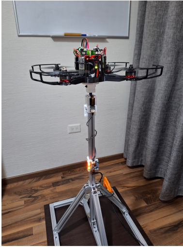
Fig. 2: The quadrotor under force-torque tests
