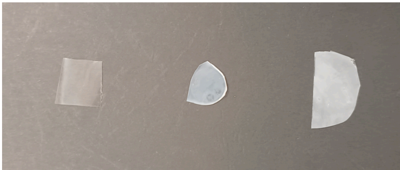
Fig. 1. Photographs of the neat P(VDF 80 -TrFE 20 ) film (from left to right): blade-casted, annealed at 120 °C and hot pressed.
