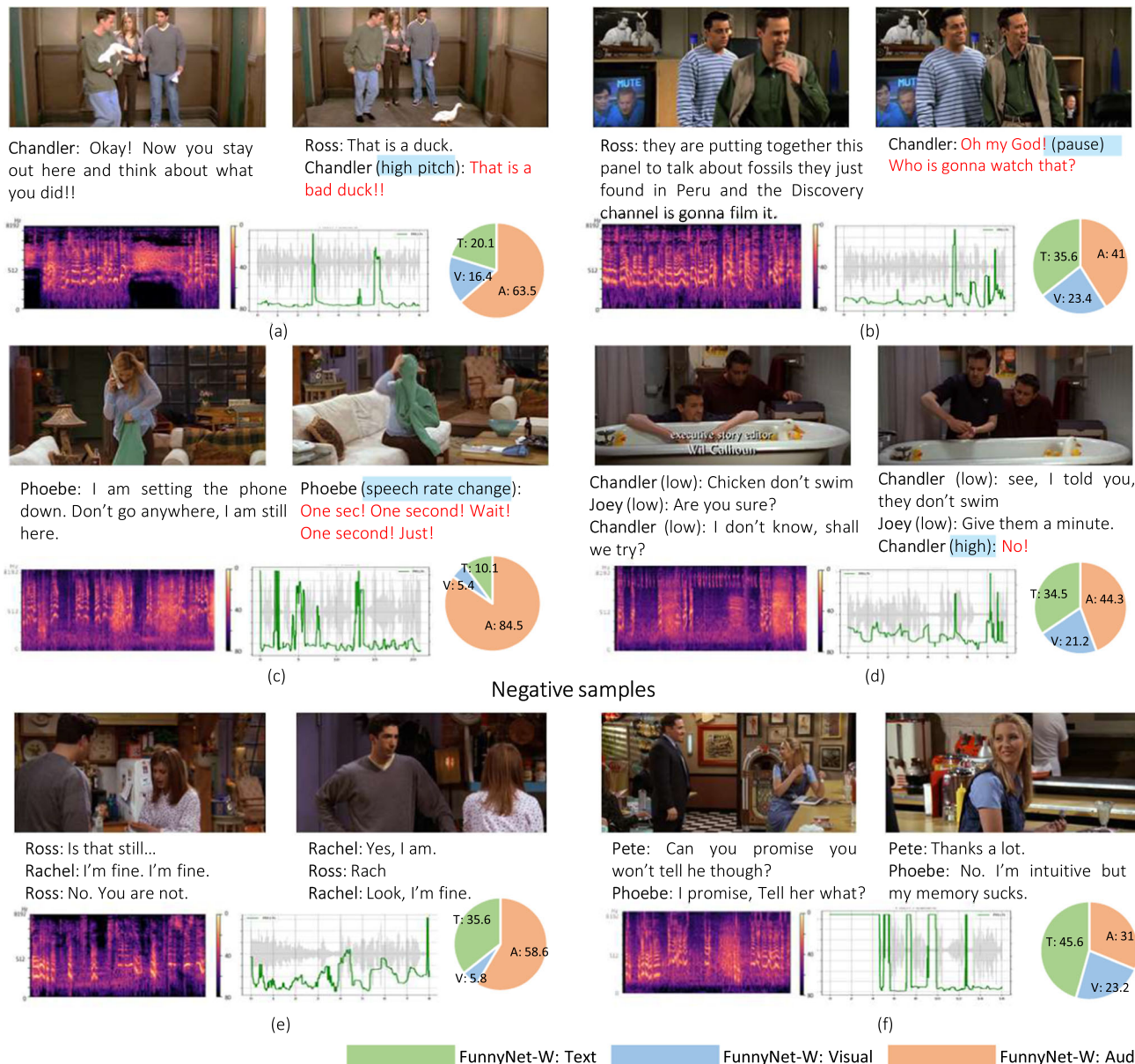
Fig. 7 Visualization of (a–d) funny, (e,f) non-funny predictions on the Friends test set. We show the audio, visual and text inputs, the learned average weights of cross-attentions from CAF (pie chart), and the subtitles (for better understanding) (Color figure online)
