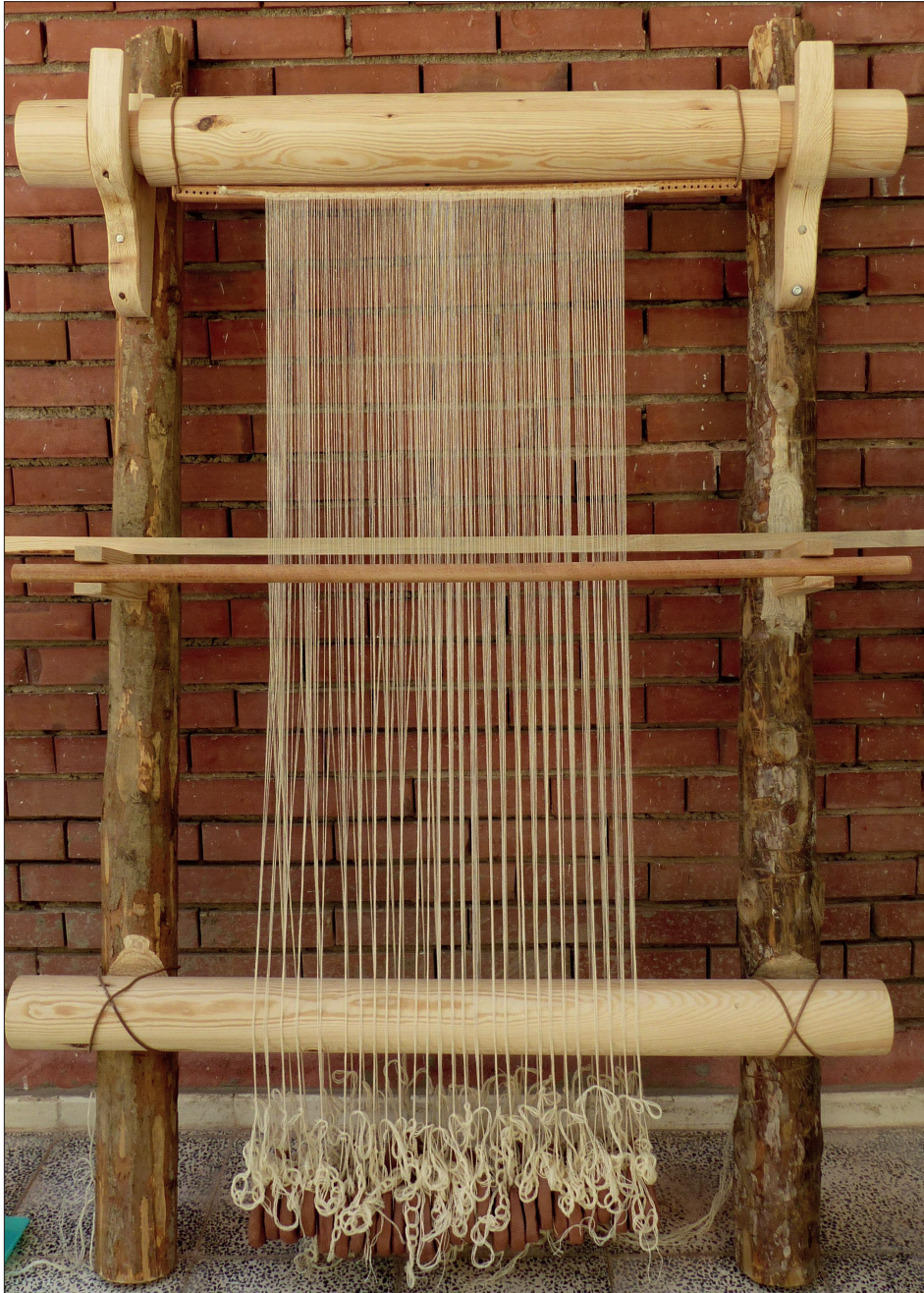
➤ Fig. 1. Warp weighed vertical loom reconstructed from the loom weights found at Kültepe. Reconstruction by Eva Andersson Strand, Fikri Kulakoğlu and Cécile Michel within the project The fabric of memory: Kültepe, a test laboratory for interdisciplinary research (dir. C. Michel), LabEx Past in Present.
