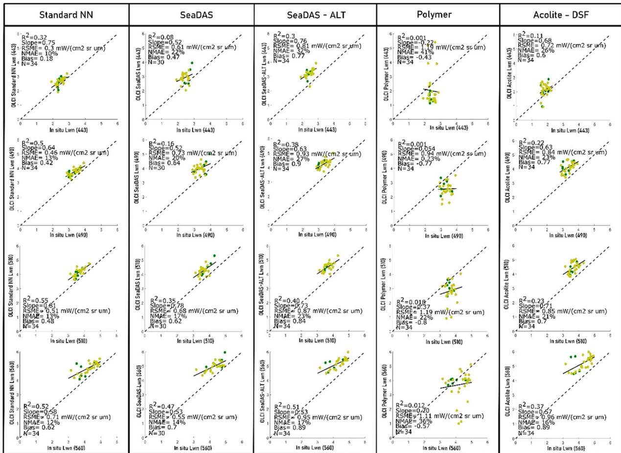
FIGURE 5 Scatterplots of the match-up exercise of the atmospheric correction algorithm (AC) retrieval and the in situ  $L_{wn}$  (443, 490, 510, 560 nm). Colors indicate the OWT: OWT 3 in green, OWT 4 in yellow.
