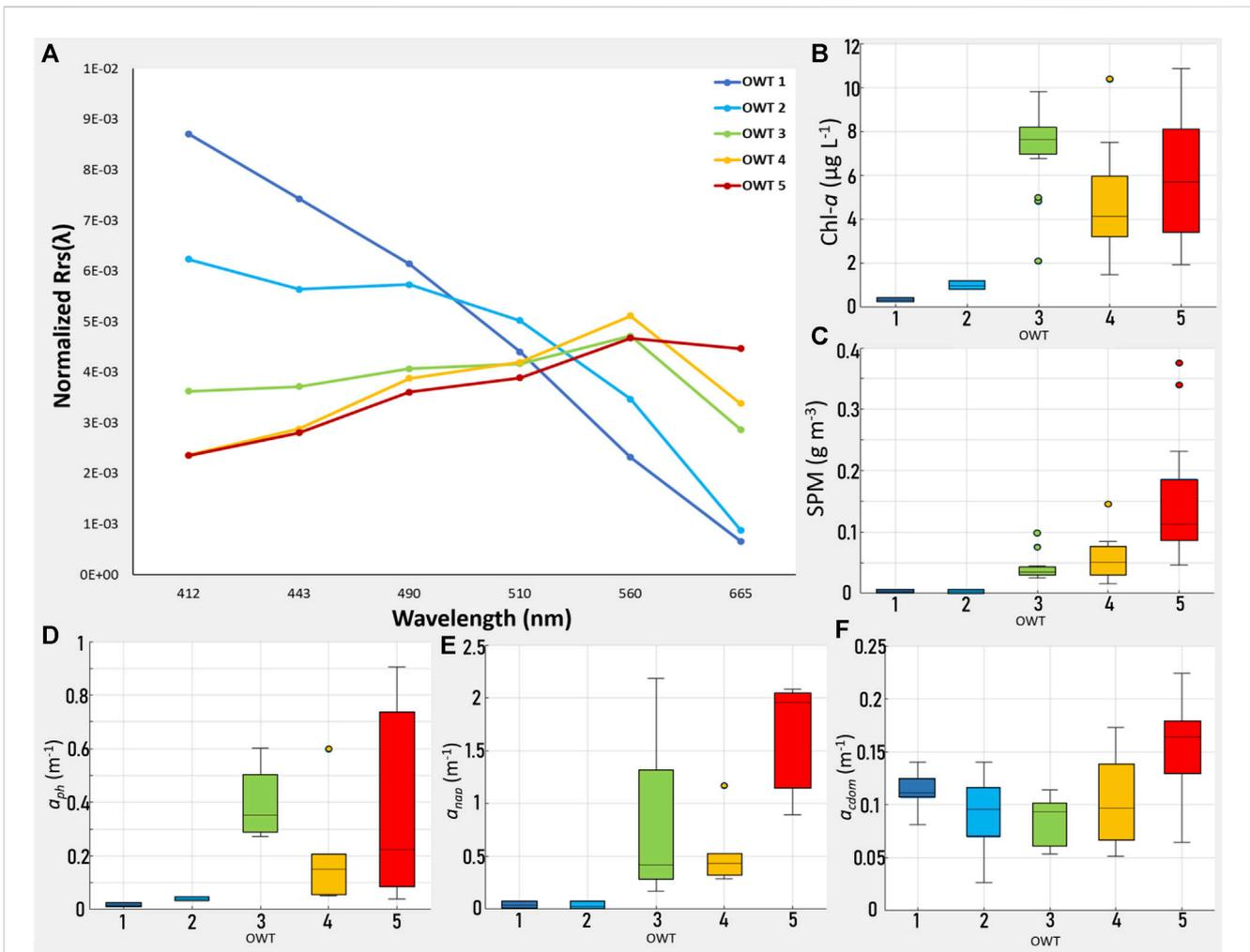
FIGURE 3 (A) Averaged normalized ( $R_{rs}(\lambda)$ ) spectra corresponding to the OWTs; box plots illustrating the distribution of Chl- $a$  ( $\mu\text{g L}^{-1}$ , (B), SPM ( $\text{g m}^{-3}$ , (C),  $a_{ph}$  (443,  $\text{m}^{-1}$ , (D),  $a_{nap}$  (443,  $\text{m}^{-1}$ , (E),  $a_{cdom}$  (443,  $\text{m}^{-1}$ , (F).
