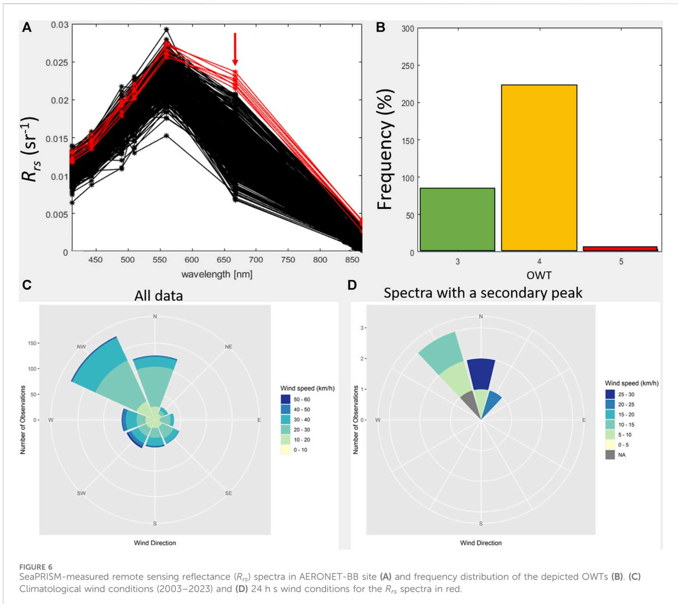
FIGURE 6 SeaPRISM-measured remote sensing reflectance ( $R_{rs}$ ) spectra in AERONET-BB site (A) and frequency distribution of the depicted OWTs (B). (C) Climatological wind conditions (2003–2023) and (D) 24 h s wind conditions for the  $R_{rs}$  spectra in red.
