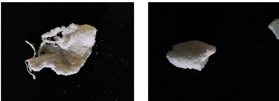
Figure 24. photos of some of the agglomerates recovered from the reactions with the poisons.
