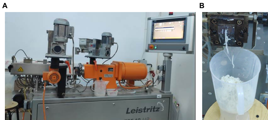
Figure S1. Photos of the (A) twin screw extruder used for the extrusion of the PVA/Fibers mixture, and (B) aspect of the extruded product at the exit of the die.
