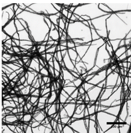
Figure S3: Optical micrograph of an aqueous suspension of neat cellulose fibers.
