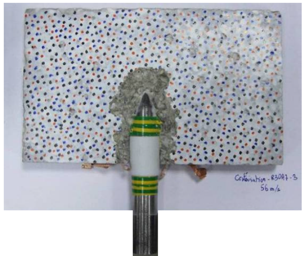
Fig. 12 Final damage state of the tile tested with the long projectile launched at 56 \text{ ms}^{-1}
