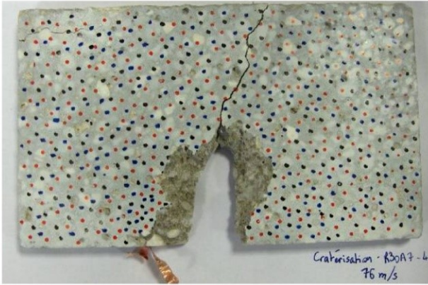
Fig. 9 Final damage state of the tile tested with the short projectile launched at 76 \text{ ms}^{-1}
