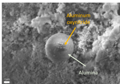
(a) Scanning electron microscope image of a large micrometric alumina particle with an aluminum oxynitride inclusion. O_2 -21% / N_2 -79%, 1 bar.
