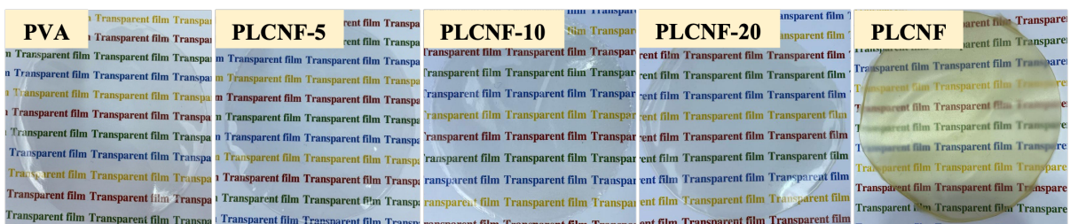
Fig SI3. Photographs of neat PVA, PLCNF, and PVA/PLCNF composite films with different PLCNF concentrations (0, 5, 10, 15, and 20 wt%).
