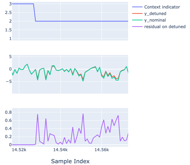
Fig. 5. Zoomed view of Fig. 4 around the region where the anomaly is introduced showing the kind of error on the time evolution to be detected through normality characterization.
