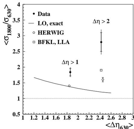
FIG. 1. The ratio of the dijet cross sections at  $\sqrt{s} = 1800$  and 630 GeV for  $\Delta\eta > 1$  and  $\Delta\eta > 2$ . The inner error bars on the data points represent statistical uncertainties; the outer bars represent statistical and uncorrelated systematic uncertainties added in quadrature. The error bars on the HERWIG predictions represent statistical uncertainties. The LO and BFKL predictions are analytical calculations.
