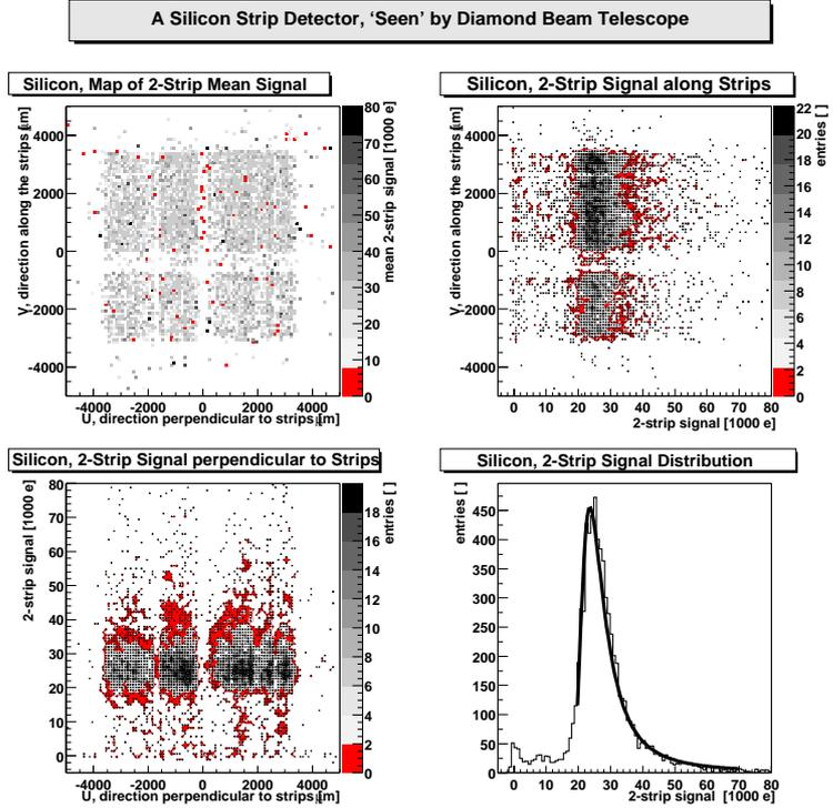
Fig. 9. Signal distribution in a silicon strip detector plane. The signals were measured on the two strips nearest to the track (“transparent” analysis). The tracks were reconstructed by the diamond beam telescope.
