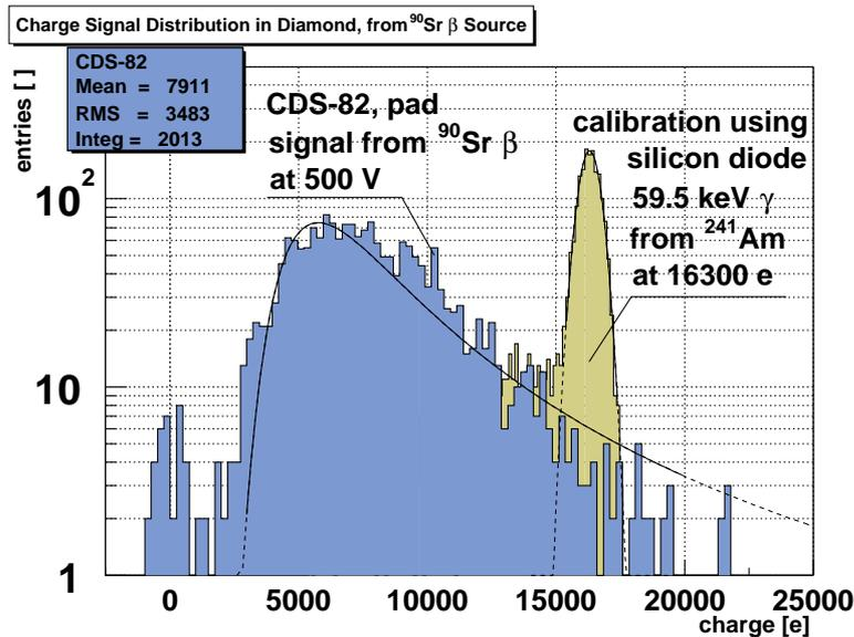
Fig. 2. Foreground: distribution of the charge measured on a solid electrode in one of the diamond planes using electrons from a  $^{90}\text{Sr}$   $\beta$ -source. Background: distribution of the charge signal from a silicon diode using  $59.5 \text{ keV}$  photons from  $^{241}\text{Am}$ . The same electronic amplification channel was used.
