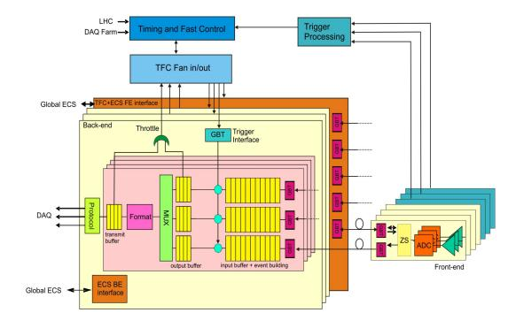
**Figure 1:** The readout scheme of the upgraded LHCb detector. The front-end is at the right and sends its data to the TELL40 boards which are the main pieces of the new DAQ design. The outputs of the TELL40 are cupper cables connected to a large switch which dispatches the data to the event filter farm.
