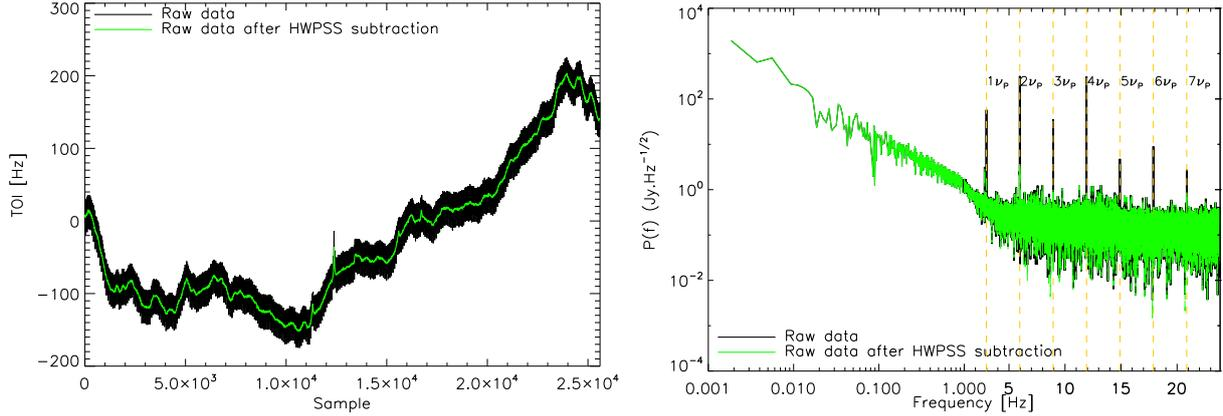
**Fig. 4.** TOI (*left*) and power spectrum (*right*) of an observation of Orion OMC-1 for a single KID. Raw data are presented in black and the Half Wave Plate systematic signal (HWPSS) subtracted data in green.
