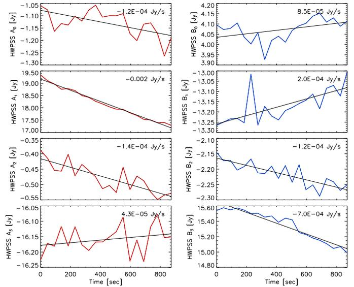
**Fig. 5.** Absolute amplitudes of the four main harmonics of the HWPSS as a function of time. Each point is a measurement of these amplitudes on a chunk of approximately 30 s. The amplitudes show a slow and linear drift in time.
