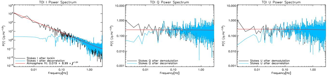
**Fig. 6.** From left to right: power spectra of the Stokes  $I$ ,  $Q$ , and  $U$  pure TOIs (black) after applying the lock-in procedure to the raw data in Fig. 4. A bandpass filter ([0.01, 2.9] Hz) was applied to reject any high-frequency noise and half wave plate systematic signal (HWPSS) residual at the fourth harmonics. In blue we also show the power spectra after applying the decorrelation procedure to the demodulated data. See Sect. 4.4 for details.
