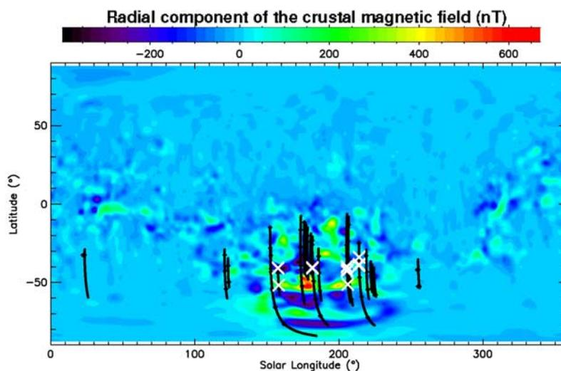
**Figure 3.** Trajectories of Mars Express during nadir viewing observations by SPICAM UVS. Only the part of each orbit with the spacecraft below 1000 km in altitude has been plotted. These trajectories are plotted on a 2-D map of the radial component of the Martian magnetic crustal field as calculated at 200 km in altitude [Purucker *et al.*, 2000]. The positions of the identified aurora during these nadir viewing orbits are also plotted with white crosses.
