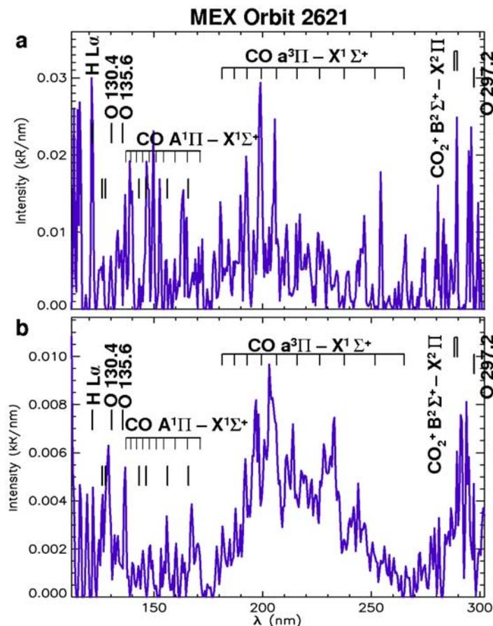
**Figure 1.** SPICAM ultraviolet spectrograph (UVS) spectra of the aurora event during orbit 2621. (a) As measured with the spatial bins facing the narrow part of the slit (best spectral resolution) during 14 s. (b) As measured with the spatial bins facing the large part of the slit (lowest spectral resolution). Each spectrum is the average of the 28 individual spectra measured during this event on the two spatial bins (14 each) either with the worst spectral resolution or the best one.
