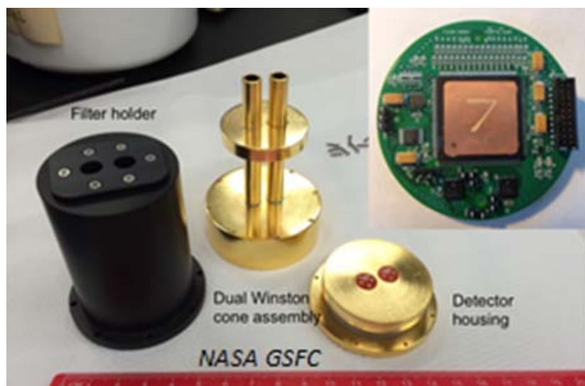
Fig. 5. NASA GSFC is testing early engineering models of the critical components the NFR. Dual Winston cone assembly and thermopile FEE readout (diameter \sim 70 mm) that uses a GSFC rad-hard mixed-signal ASIC (NASA GSFC).
