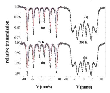
Figure 3. <sup>57</sup>Fe Mössbauer spectra recorded on bare (a) and hybrid (b) particles at 77 (left side) and at 300 K (right side)
