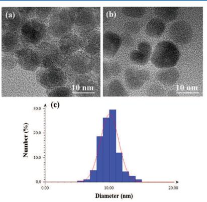
Figure 4. TEM images of the as-produced maghemite particles (a) and their related nanohybrids resulting from DA grafting (b). The size distribution of the iron oxide particles, as inferred from SAISAM program, is given for indication (c).
