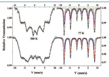
Figure 5. Fe Mossbauer spectra of the as-produced maghemite particles (bottom) and their related nanohybrids resulting from DA grafting (top) recorded at 300 (left) and 77 K (right).
