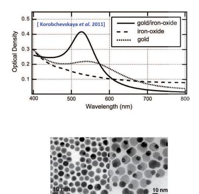
Figure 5.6: UV-vis spectra of the gold, iron oxide and iron oxide/gold as well as the transmission electron microscopy images of Au (left) and gold/iron oxide nanocrystals (right) from [Korobchevskaya *et al.* 2011].
