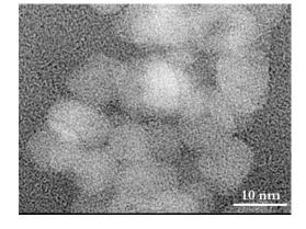
Figure 1. TEM image of the polyol-made  $\gamma\text{-}Fe_2O_3$  NPs.
