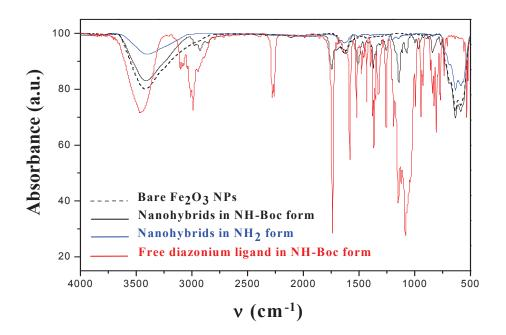
Figure 2. FTIR spectrum of NP-C<sub>6</sub>H<sub>4</sub>-C<sub>2</sub>H<sub>4</sub>-NH<sub>2</sub> compared to those of bare NPs and free diazonium salts, namely  $[BF_4, ^+N_2-C_6H_4-C_2H_4-NH-Boc]$  and  $[BF_4, ^+N_2-C_6H_4-C_2H_4-NH_2]$ .
