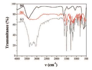
Figure 3. FTIR spectra of the as-produced maghemite particles (a) and their related nanohybrids resulting from DA grafting (b) compared with that of free DA (c).
