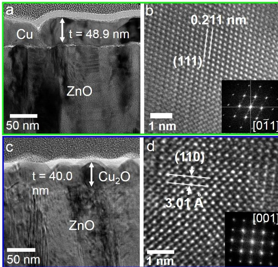
**Figure 3.4.** Cross-section TEM micrographs of the Cu (a) and the  $\text{Cu}_2\text{O}$  (c) films. HRTEM micrographs of the Cu (b) and the  $\text{Cu}_2\text{O}$  (d) films; the corresponding FFT patterns are shown at the inset.
