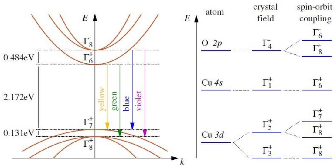
**Figure 1.2.** Schematic of the  $\text{Cu}_2\text{O}$  band structure at the  $\Gamma$ -point of the Brillouin zone, the different electronic transitions leading to the four excitonic series are indicated. Origin of conduction and valence bands from the atomic orbitals and the band splitting considering crystal-field and spin-orbit interaction are depicted on the right [17].
