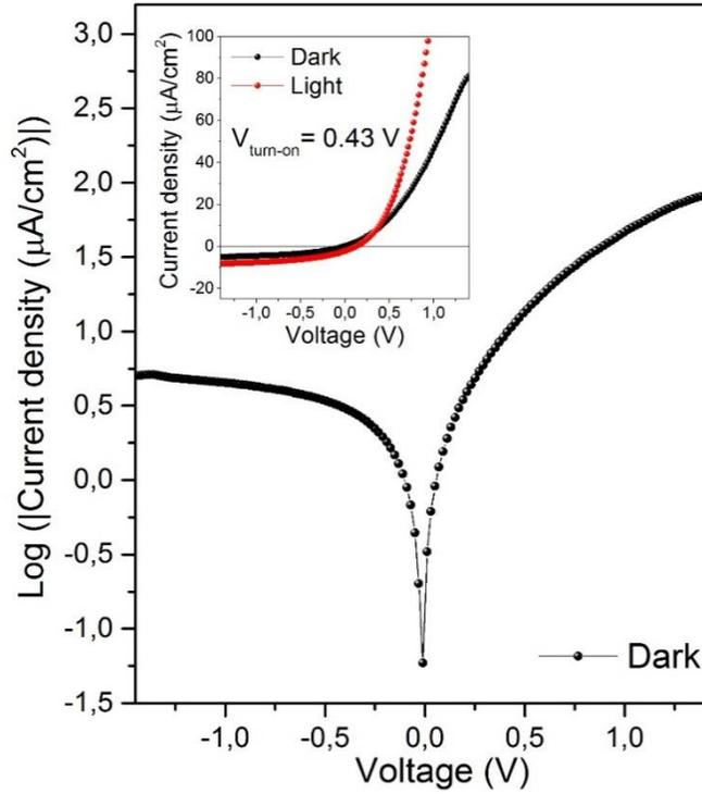
**Figure 4.6.** Current density characteristics (semi-log scale) for the Cu/ZnO Schottky junction, in the inset the I-V characteristics is shown in linear scale together with the J-V curve under illumination (red line).
