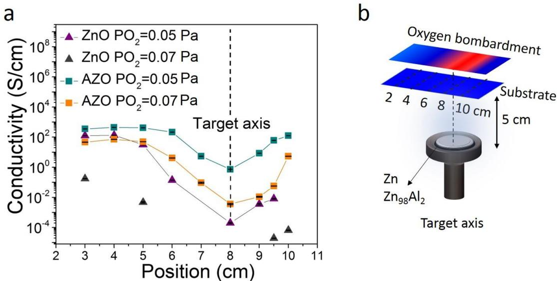
**Figure 3.2.** Conductivity of the ZnO and AZO films as a function of the position in the sputtering chamber and O<sub>2</sub> partial pressure (a). Schematic of the configuration used for the deposition and of the flux of high energetic O atoms and O<sup>-</sup> ions (b). Remark: the conductivity of sample deposited using  $P_{O_2} = 0.07$  Pa was too high to be measured near the target axis, explaining why symbols were selected instead of connecting lines in (a) for this condition.
