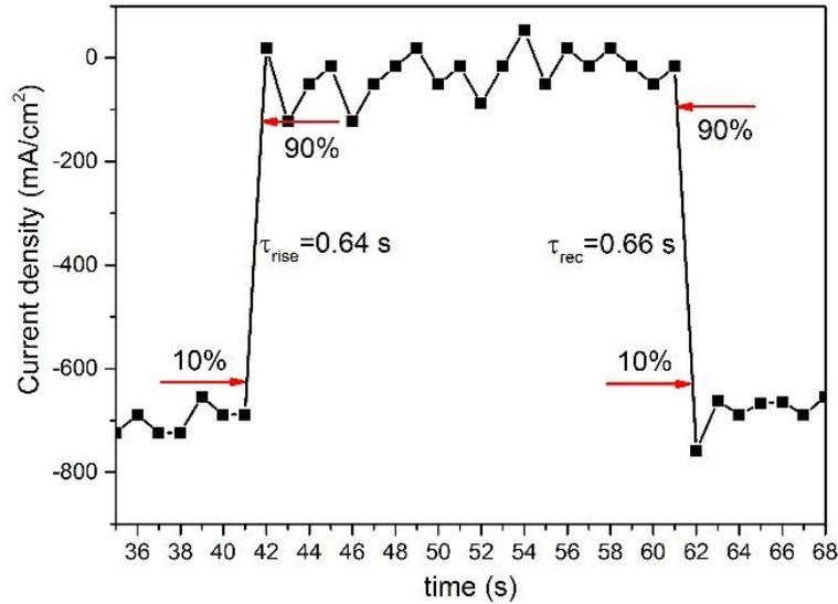
**Figure 4.9.** Current density vs. time for the Cu NP/ZnO deposited at 1500 ALD cycles, under dark/light cycles of 20 s.
