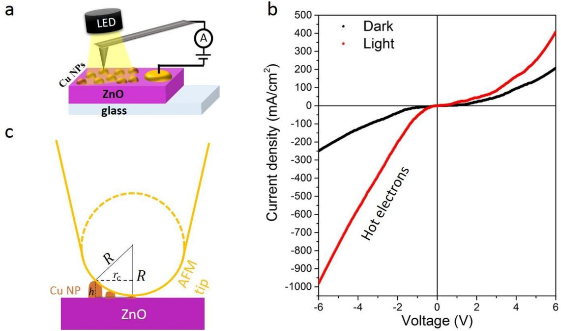
**Figure 4.7.** Photoresponse of Cu NP under visible light. Schematic of the C-AFM measurements (a). Current density characteristics of the Cu NP/ZnO device in the dark and under visible-light illumination, with an estimated contact area of  $4.3 \times 10^3 \text{ nm}^2$  (b). Schematic of the contact area between the AFM tip and the sample surface (c).
