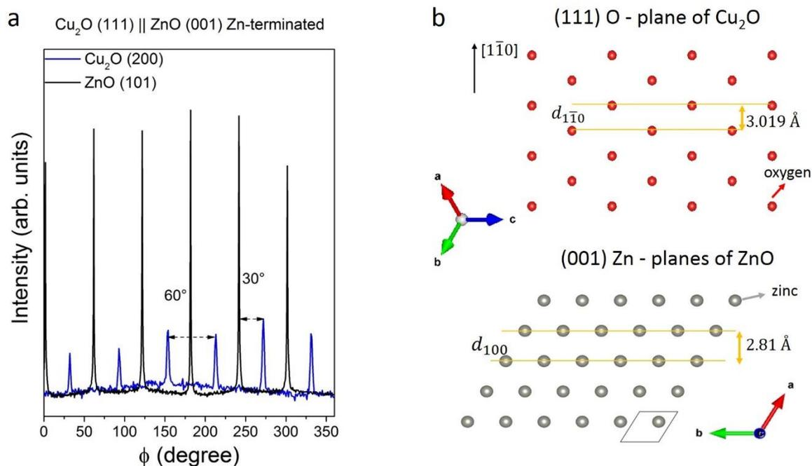
**Figure 3.13.**  $\phi$ -scan of the  $\text{Cu}_2\text{O}$  (200) and the ZnO (101) crystallographic planes of the  $\text{Cu}_2\text{O}$ -(111)/ZnO-(001)-Zn terminated sample, in logarithmic scale (a). Schematic of the oxygen atoms at the (111) planes of  $\text{Cu}_2\text{O}$  (top) and the zinc atoms at the (001) plane in ZnO (bottom) (b).
