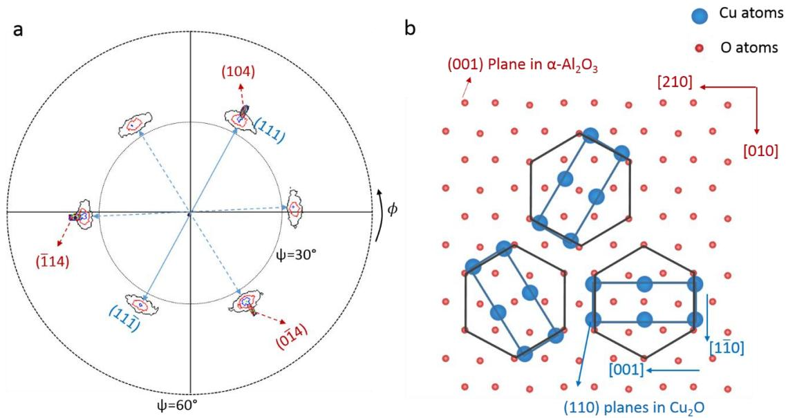
**Figure 3.9.** Pole figure of a Cu<sub>2</sub>O film deposited on  $\alpha$ -Al<sub>2</sub>O<sub>3</sub> at  $2\theta=36.42^\circ$ , the {111} and {104} family of planes for Cu<sub>2</sub>O and  $\alpha$ -Al<sub>2</sub>O<sub>3</sub>, respectively, are indicated (a). Schematic of the epitaxial relationship between the Cu<sub>2</sub>O films and the  $\alpha$ -Al<sub>2</sub>O<sub>3</sub> substrate, the different configuration, associated with the three Cu<sub>2</sub>O domains are indicated (b).
