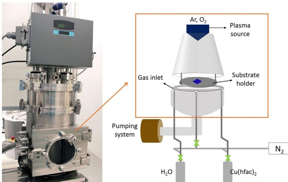
**Figure 2.6.** Picture of the ALD PICOSUN™ R-200 Advanced reactor (a). Simplified schematic of the ALD reactor, showing the reaction chamber, the plasma source at the top, and the precursor bottle and connections with the chamber at the bottom (b).
