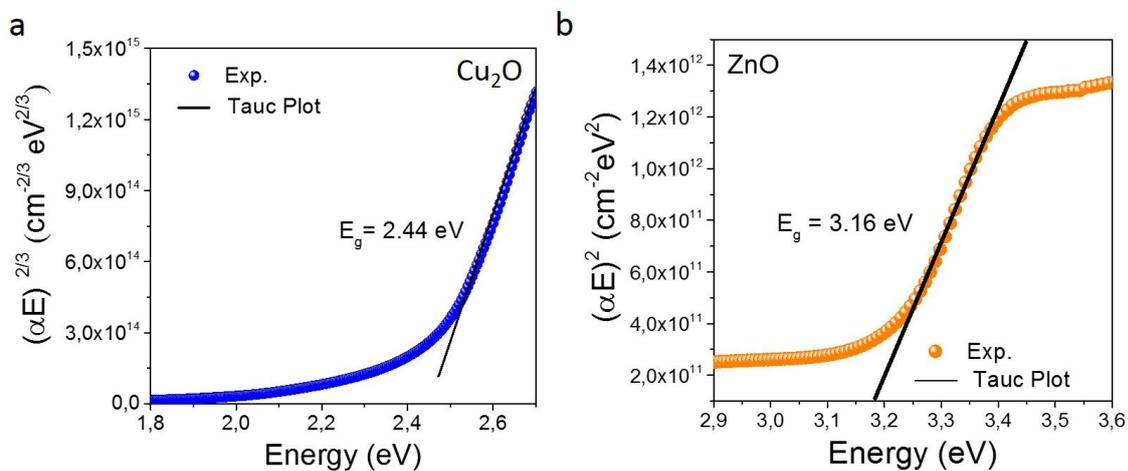
**Figure 5.7.** Tauc Plot for the Cu<sub>2</sub>O (a) and ZnO (b) films deposited on  $\alpha$ -Al<sub>2</sub>O<sub>3</sub>, and glass substrates, respectively.
