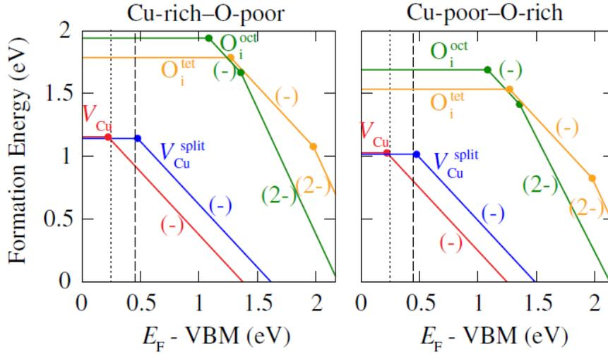
**Figure 1.3.** Theoretical calculations of the formation energy for the different acceptor levels in  $\text{Cu}_2\text{O}$ , under Cu-rich (left) and Cu-poor (right) conditions (color lines). The vertical dashed lines represent experimental values obtained from deep-level transient spectroscopy measurements [19].
