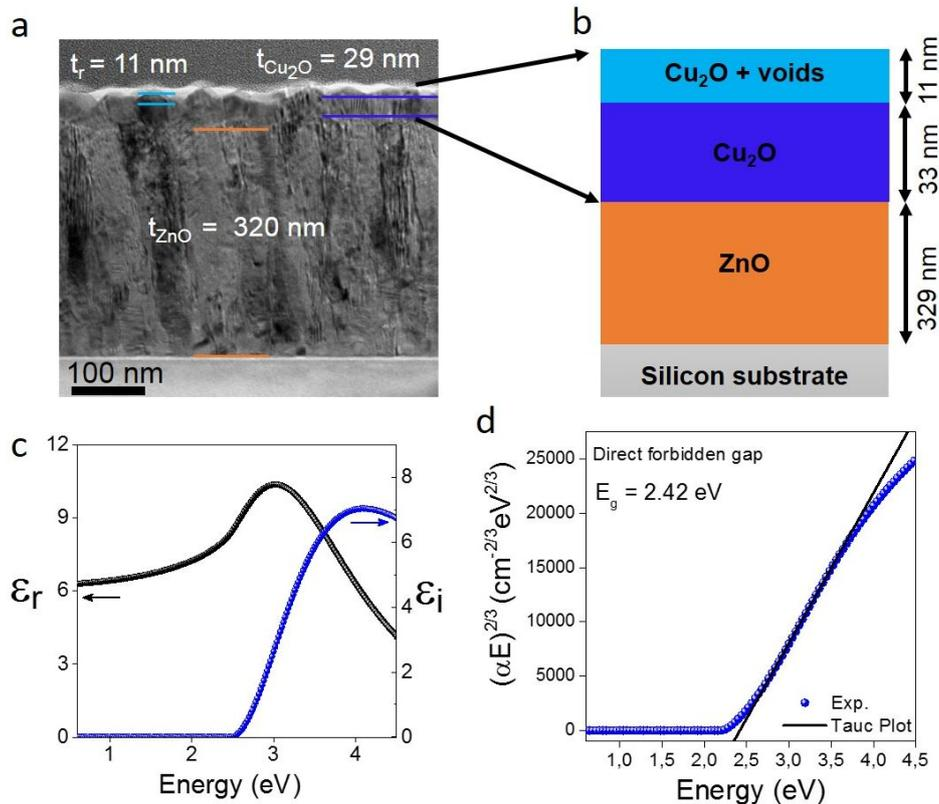
**Figure 5.5.** TEM micrograph of the  $\text{Cu}_2\text{O}/\text{ZnO}$  heterojunction (a). Schematic of the physical model used for fitting the ellipsometric data (b). Real and imaginary parts of the dielectric function of the  $\text{Cu}_2\text{O}$  film determined by ellipsometry (c). Tauc Plot for the  $\text{Cu}_2\text{O}$  film (d).
