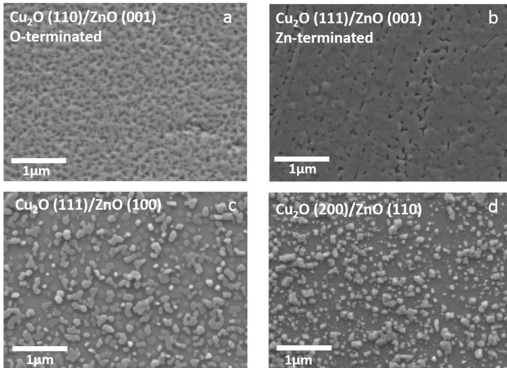
**Figure 3.11.** Top-view SEM micrographs of the Cu<sub>2</sub>O films deposited on the c-plane O-terminated (a) and Zn-terminated (b) ZnO polar substrates, and the a-plane (c) and m-plane (d) ZnO non-polar substrates.
