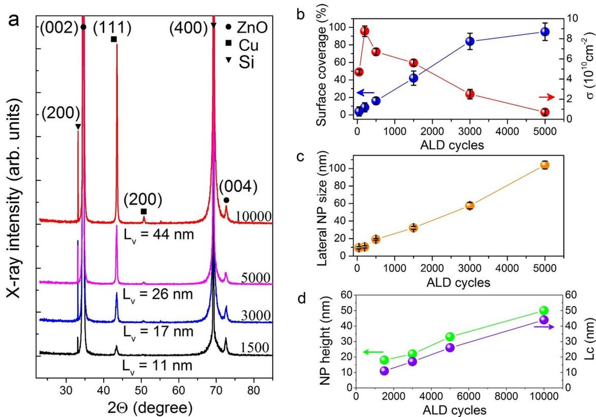
**Figure 4.2.** X-ray diffractograms of the Cu NP after 1500 (black), 3000 (blue) and 5000 (magenta) ALD cycles and the Cu film (red) deposited at 10000 ALD cycles (a). Surface coverage, density (b) and average lateral NP size (c), versus the number of ALD cycles. Average NP height (green), and coherence length (violet), versus the number of ALD cycles (d).
