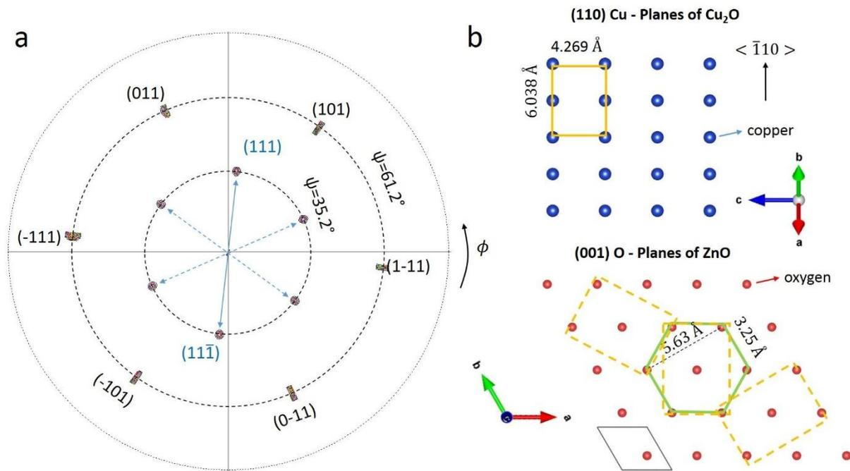
**Figure 3.12.** Pole figure of the Cu<sub>2</sub>O film deposited on ZnO at  $2\theta=36.42^\circ$ , the  $\{111\}$  and  $\{101\}$  family of planes for Cu<sub>2</sub>O and ZnO, respectively, are observed (a). Schematic of the Cu atoms at the (110) planes of Cu<sub>2</sub>O (top), and the oxygen atoms at the (001) planes of ZnO (bottom). The different configuration in which the Cu<sub>2</sub>O domains can grow on top of the ZnO substrate (b).
