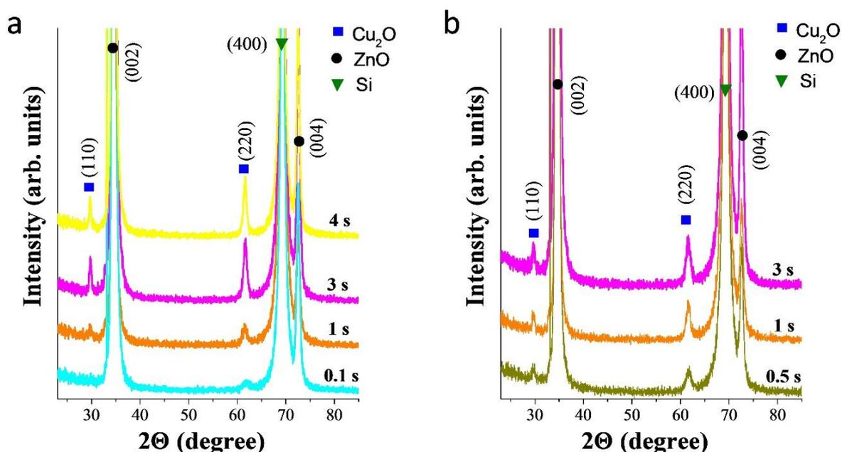
**Figure 2.7.** Optimization of the precursors pulse length:  $\text{H}_2\text{O}$  (a) and  $\text{Cu}(\text{hfac})_2$  (b) for the deposition of  $\text{Cu}_2\text{O}$  on  $\text{ZnO}$  substrates. The substrate temperature and the number of cycles were fixed at  $280^\circ\text{C}$  and 5000, respectively.
