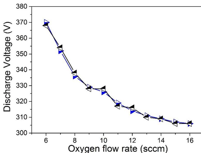
**Figure 2.11.** Evolution of the discharge voltage as a function of the oxygen partial pressure.
