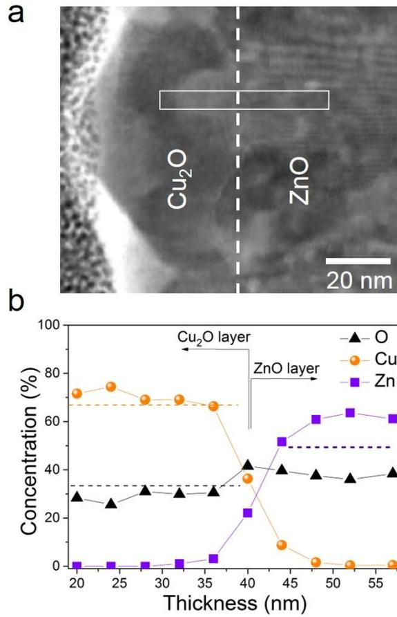
**Figure 5.4.** Bright field STEM micrograph taken at the interface between  $\text{Cu}_2\text{O}$  and  $\text{ZnO}$  films (a). Composition profiles obtained by EDS in the region enclosed by a rectangle in a (dashed lines indicate the expected Cu, Zn and O concentrations for the stoichiometric  $\text{Cu}_2\text{O}$  and  $\text{ZnO}$ ) (b).
