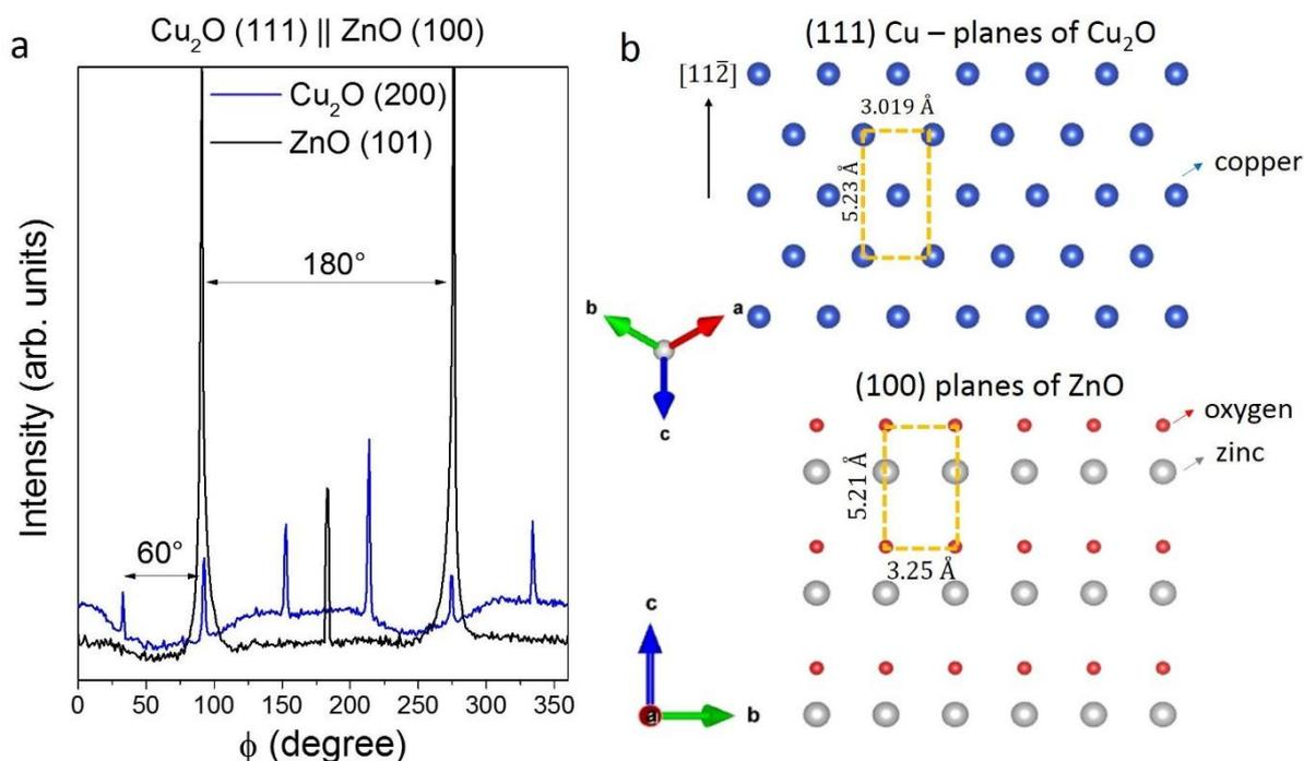
**Figure 3.14.**  $\phi$ -scan of the  $\text{Cu}_2\text{O}$  (200) and the ZnO (101) crystallographic planes of the  $\text{Cu}_2\text{O}$ -(111)/ZnO-(100) sample, in logarithmic scale (a). Schematic of the Cu atoms at the (111) planes of  $\text{Cu}_2\text{O}$  (top) and the Zn atoms at the (100) plane in ZnO (bottom) (b).
