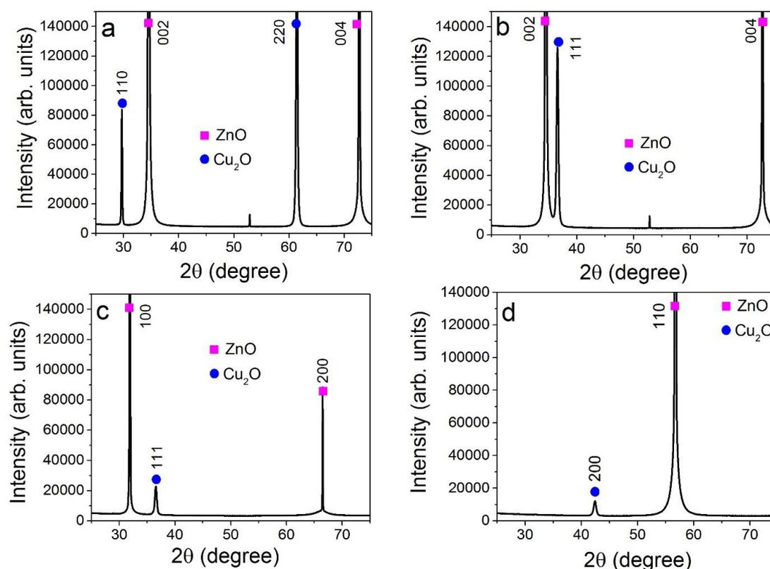
**Figure 3.10.** X-ray diffractograms of the  $\text{Cu}_2\text{O}$  films deposited on c-plane oriented O-terminated ZnO (a), c-plane oriented Zn-terminated ZnO (b), a-plane ZnO (c), and m-plane ZnO (d) substrates.
