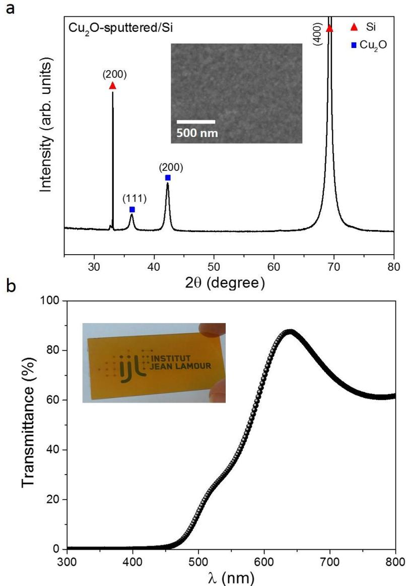
**Figure 5.11.** X-ray diffractogram of the  $\text{Cu}_2\text{O}$  film deposited on Si substrate (a), a top-view SEM micrograph is shown as inset. Transmittance spectrum of the  $\text{Cu}_2\text{O}$  film deposited on a glass substrate (b), a picture of the sample is shown as inset.
