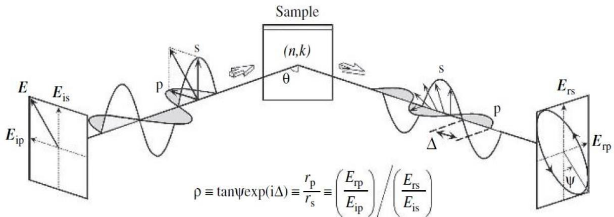
**Figure 2.14.** Configuration for spectroscopic ellipsometry measurements [143].
