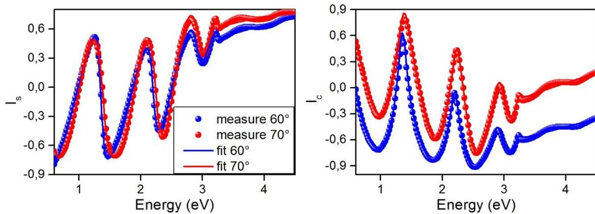
**Figure V.** Measured and simulated ellipsometric spectra for the Cu<sub>2</sub>O/ZnO films at 60° (blue) and 70° (red).
