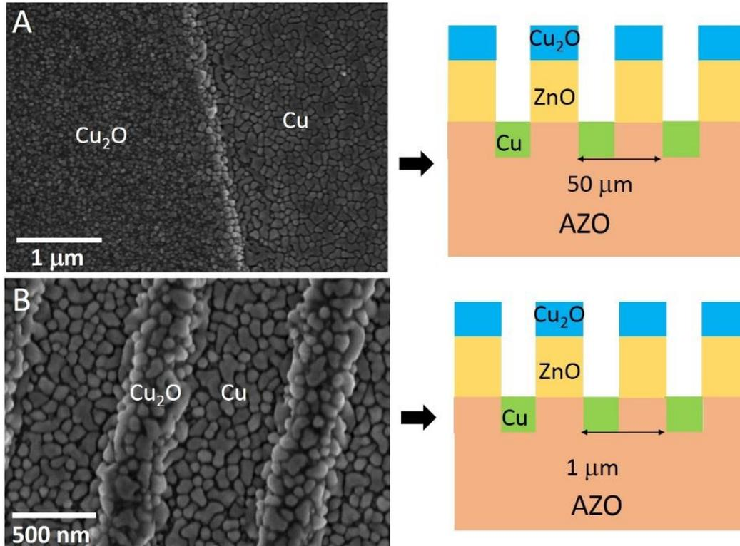
**Figure 3.21.** Cu<sub>2</sub>O and Cu area-selective deposition on features of different sizes: 50 μm (a) and 1 μm (b).
