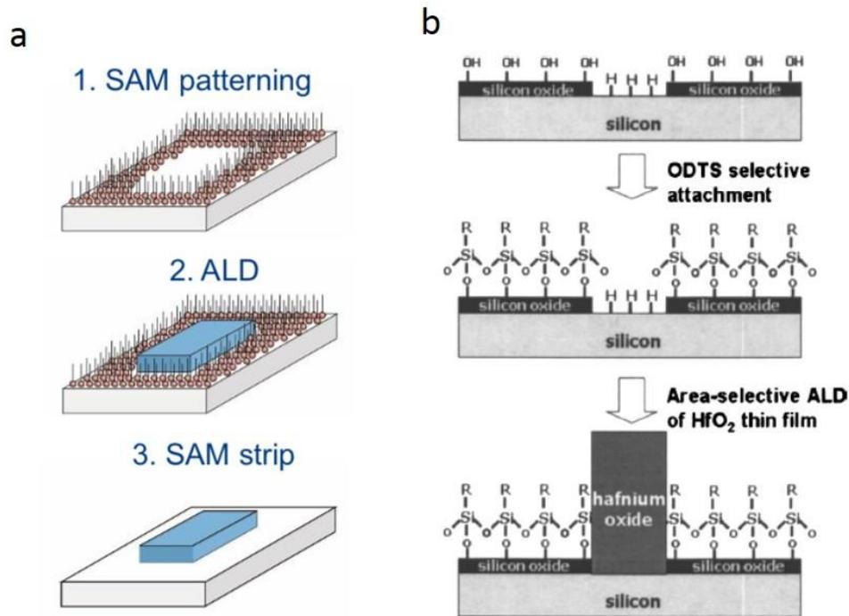
**Figure 3.1.** Schematic of the AS-ALD process by deactivation of the surface using SAMs [1] (a). Schematic of the AS-ALD process for the fabrication of  $\text{HfO}_2$  using octadecyltrichlorosilanes (ODTS) SAMs to modify the surface [165].
