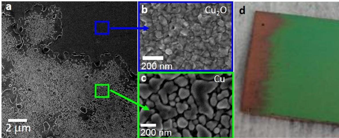
**Figure 3.6.** Top-view SEM micrographs of the sample composed of a mixture between  $\text{Cu}$  and  $\text{Cu}_2\text{O}$  (a). Amplified micrograph at the  $\text{Cu}_2\text{O}$  (b) and  $\text{Cu}$  (c) regions. Picture of the sample, where the interface between the  $\text{Cu}$  (orange) and the  $\text{Cu}_2\text{O}$  (green) can be observed (d).
