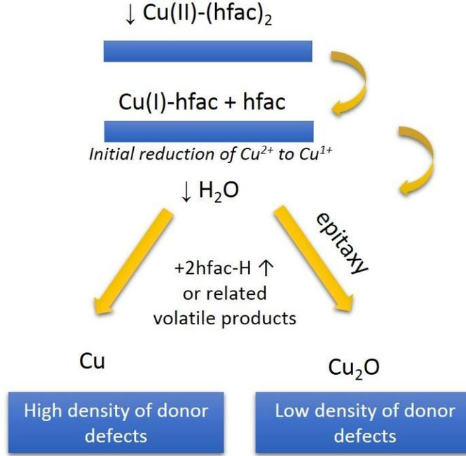
**Figure 3.17.** Schema illustrating the mechanism behind the selective deposition of Cu and Cu<sub>2</sub>O.
