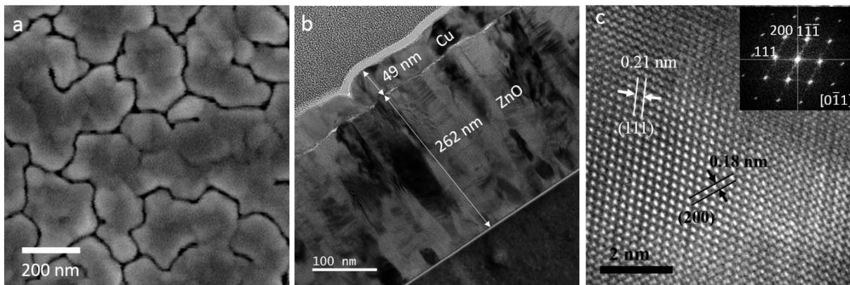
**Figure 4.4.** Top-view SEM micrographs of the Cu film after 10000 ALD cycles (a). TEM bright field micrograph taken from a cross-section of the Cu film (b). HRTEM micrograph taken to the Cu film (c) and the corresponding FFT pattern (inset).
