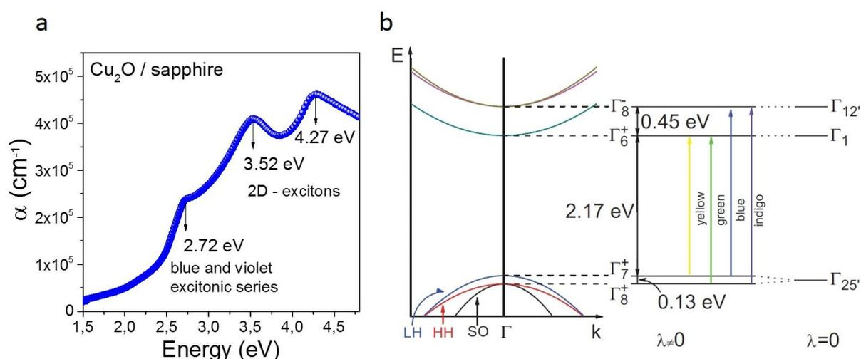
**Figure 5.6.** Absorption coefficient for the  $\text{Cu}_2\text{O}$  film deposited on  $\alpha\text{-Al}_2\text{O}_3$  (a). Schematic of the  $\text{Cu}_2\text{O}$  electronic band structure around the center of the Brillouin zone ( $\Gamma$ -point), without ( $\lambda=0$ ) and with ( $\lambda\neq 0$ ) spin-orbit interaction. Transition from the  $E_C$  to the  $E_V$  leads to the four excitonic series represented in color lines (b).
