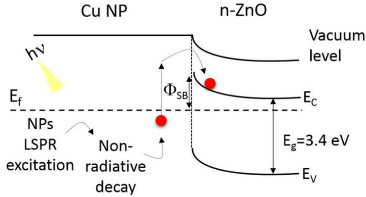
**Figure 4.10.** Schematic illustration of the energy band alignment at the Cu NP/ZnO interface together with the representation of hot electron generation at the Cu NP and the transfer to ZnO through the Schottky barrier.
