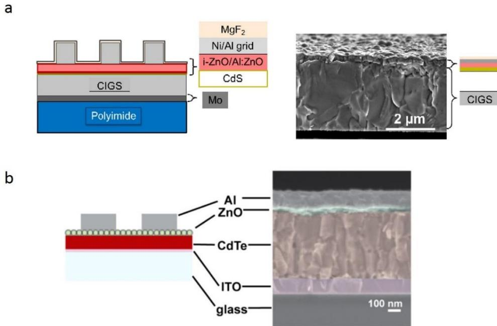
**Figure 1.7.** Schematic and cross-section SEM micrograph of a thin film CIGS solar cell on a flexible polyimide substrates, from [74] (a). Schematic and colored cross-section SEM micrograph of a CdTe solar cell, from [75] (b).
