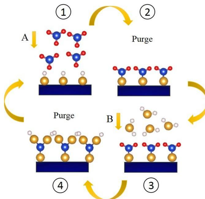
**Figure 2.1.** Schematic of an ALD four-step process: (1) exposure to the first precursor A, (2) purge step, (3) exposure to the second precursors B, and (4) final purge step.
