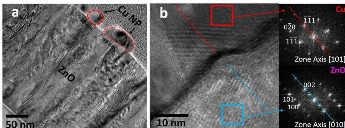
**Figure 4.3.** Bright-field-TEM micrograph of the CuNP/ZnO sample (a). High resolution TEM micrograph at the interface between the Cu NP and the ZnO film. FFT patterns taken at the Cu and ZnO regions are shown in the inset.
