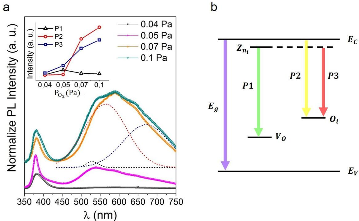
**Figure 3.16.** Normalized photoluminescence spectra of ZnO films deposited at different  $P_{O_2}$ , the evolution of the areal intensity of the defect bands with the oxygen partial pressure is presented at the inset (a). Energy level diagram illustrating the defect levels in ZnO and the transition observed in the photoluminescence spectra (b).
