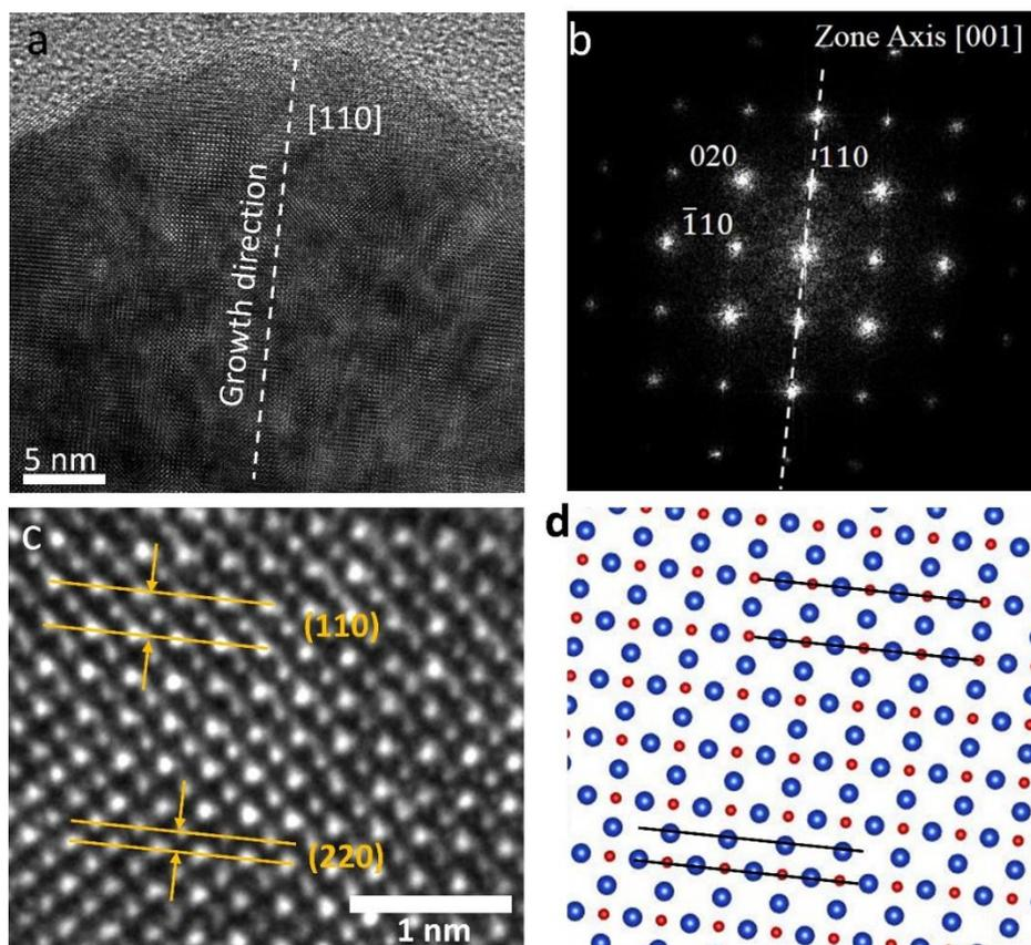
**Figure 5.3.** Cross-section HR-TEM micrograph of the  $\text{Cu}_2\text{O}$  film (a) with the corresponding FFT pattern (b). Amplified HR-TEM micrograph, the (110), and (220) planes are indicated (c). Schematic of the  $\text{Cu}_2\text{O}$  crystal structure (d).
