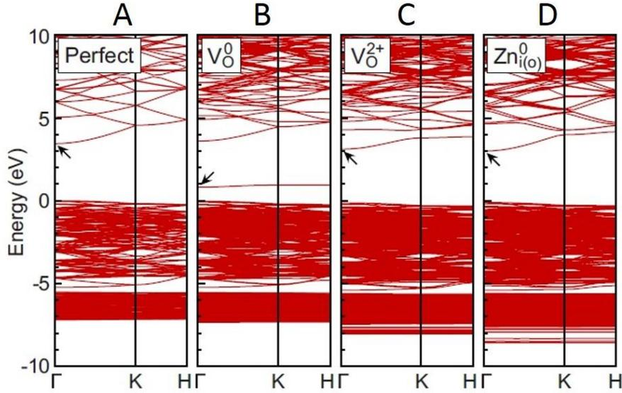
**Figure 1.5.** Band structure of a ZnO perfect crystal (A), and considering different types of defects: oxygen vacancies in the neutral state (B) and 2+ charge states (C), and Zn interstitial at the octahedral site in the neutral state [52].
