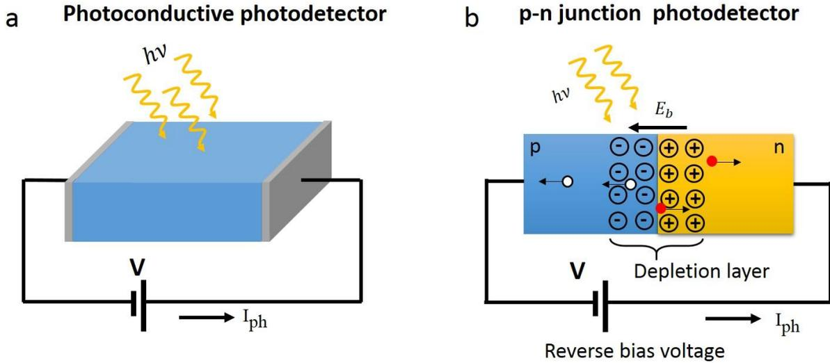
**Figure 1.15.** Schematic of a photoconductive (a) and a p-n junction (b) photodetectors.
