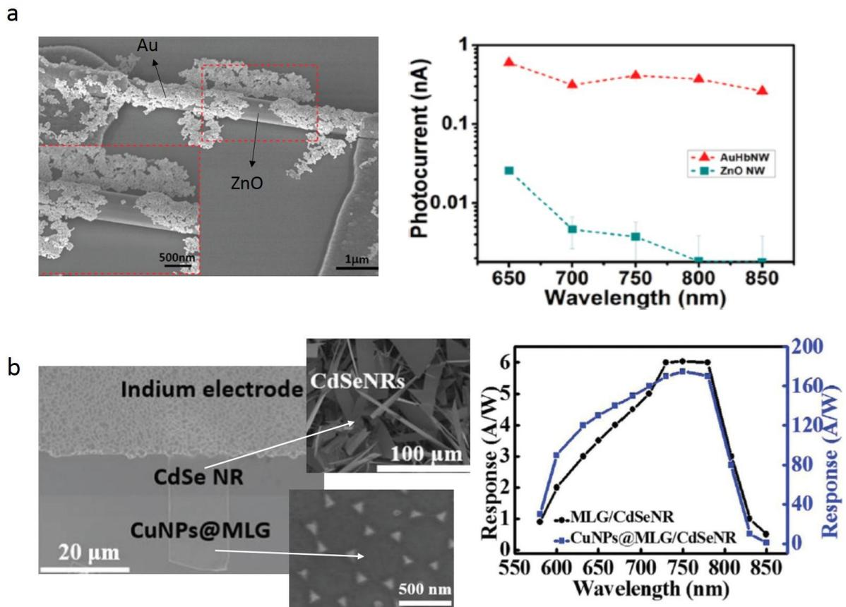
**Figure 1.17.** SEM micrograph of an hybrid photodetector made of Au nanorods on ZnO nanowires (left), the photocurrent of the hybrid device (red) and of the virgin ZnO nanowires (blue) as a function of the wavelength (right), modified from [5] (a). SEM micrograph of a MLG – CdSe nanoribbons Schottky diode, with Cu nanoparticles deposited on the MLG (left), the responsivity of the Schottky diode with (blue) and without (black) the Cu nanoparticles, modified from [120] (b).
