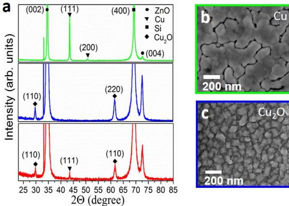
**Figure 3.3.** X - ray diffractograms of the samples after the ALD deposition at 280°C (a). Top-view SEM micrographs of the Cu film (b) and the Cu<sub>2</sub>O film (c).
