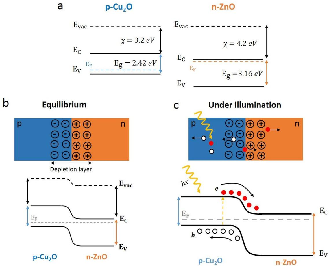
**Figure 5.10.** Band energy diagram of the isolated Cu<sub>2</sub>O and ZnO semiconductor (a) and after the formation of the heterojunction under equilibrium (b) and under illumination at 0 bias voltage (c).
