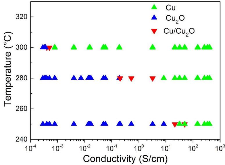
**Figure 3.7.** Diagram of the different phases deposited (Cu, Cu<sub>2</sub>O or mixture) depending on the temperature and the substrate conductivity.
