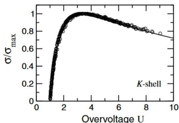
**Figure 2.19.** Normalized ionization cross-section of the K shell vs. overvoltage from [146]. The circle represent the DWBA calculation from several elements and the continuous line an analytical expression proposed by Campos *et al.*
