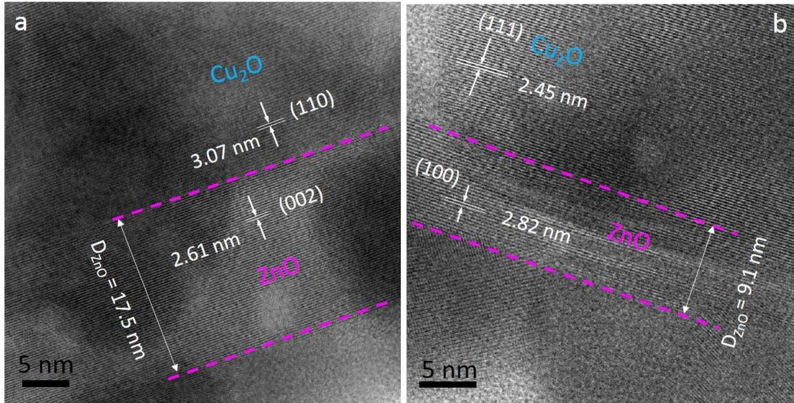
**Figure 5.17.** HR-TEM micrograph showing the orientation relationship between the  $\text{Cu}_2\text{O}$  and the ZnO nanowires.
