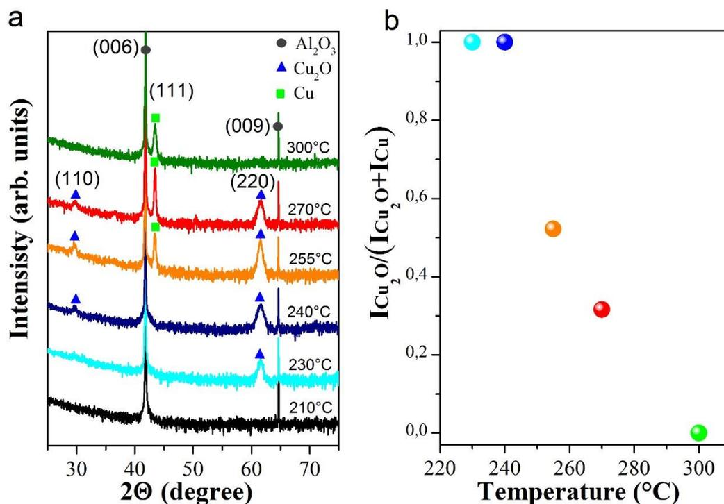
**Figure 3.8.** X-ray diffractograms Cu<sub>2</sub>O and Cu films on sapphire substrates, showing the temperature-dependent selectivity (a). Evolution of the Cu and Cu<sub>2</sub>O XRD intensity with deposition temperature (b).
