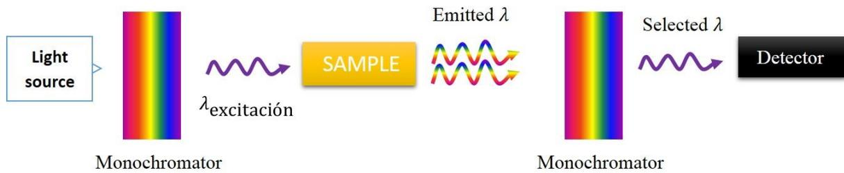
**Figure 2.16.** Schematic principle of the photoluminescence spectroscopy set-up.
