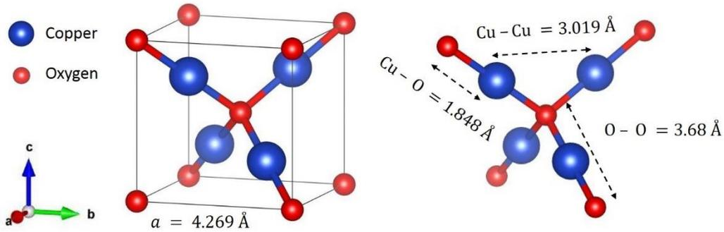
**Figure 1.1.** Crystal structure of cuprite Cu<sub>2</sub>O (space group Pn-3m). The bond lengths are indicated.
