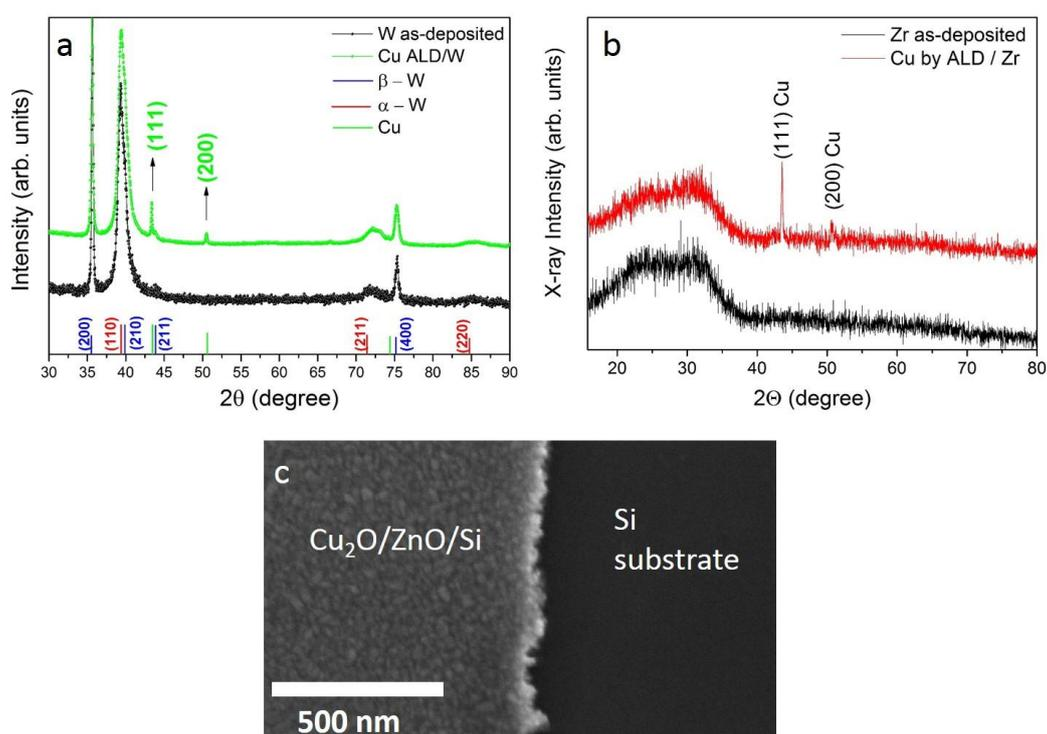
**Figure 3.18.** X-ray diffractometer of a Cu film deposited by ALD on a 200 nm W film (a) and on a 500 nm Zr film (b). Top view SEM micrograph for a  $\text{Cu}_2\text{O}/\text{ZnO}/\text{Si}$  sample showing the area-selectivity of  $\text{Cu}_2\text{O}$  on ZnO vs. Si substrates (c).
