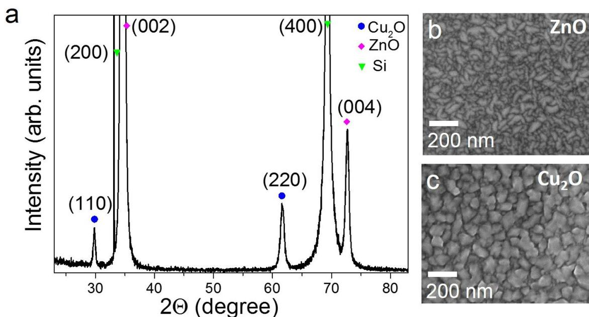
**Figure 5.1.** X-ray diffractogram of the  $\text{Cu}_2\text{O}/\text{ZnO}$  heterostructure (a). Top-view SEM micrograph of the as-grown ZnO film (b) and of the  $\text{Cu}_2\text{O}$  film deposited on top (c).
