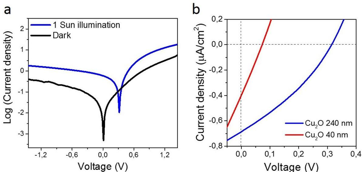
**Figure 5.13.** Current density characteristics of the heterojunction (in semi logarithmic scale) in dark (black line) and under 1 Sun illumination (blue line) (a). Current density characteristics amplified around the short-circuit current and open-circuit voltage points for the heterojunction with (blue line) and without (red line) the 240-nm-Cu<sub>2</sub>O sputtered layer (b).
