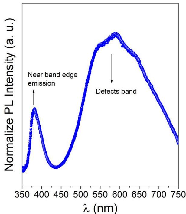
**Figure 2.17.** Photoluminescence spectrum of a typical ZnO film.
