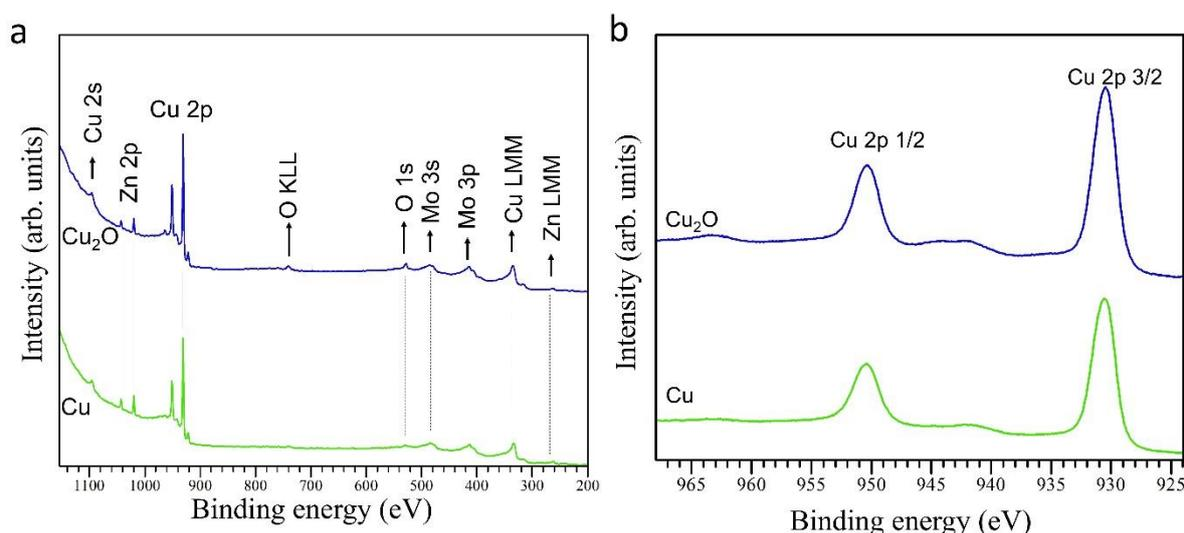
**Figure 3.15.** XPS survey scan (a) and Cu 2p spectra (b) for a Cu<sub>2</sub>O (blue) and a Cu (green) film.
