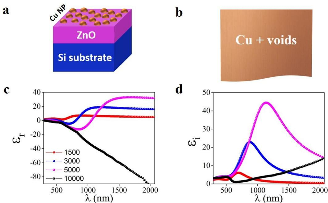
**Figure 4.5.** Schematic of the physical model used for fitting the ellipsometry data for the Cu NP (a) and the Cu film (b). Real (c) and imaginary (d) part of the dielectric function of the Cu NP and the Cu film (black line).
