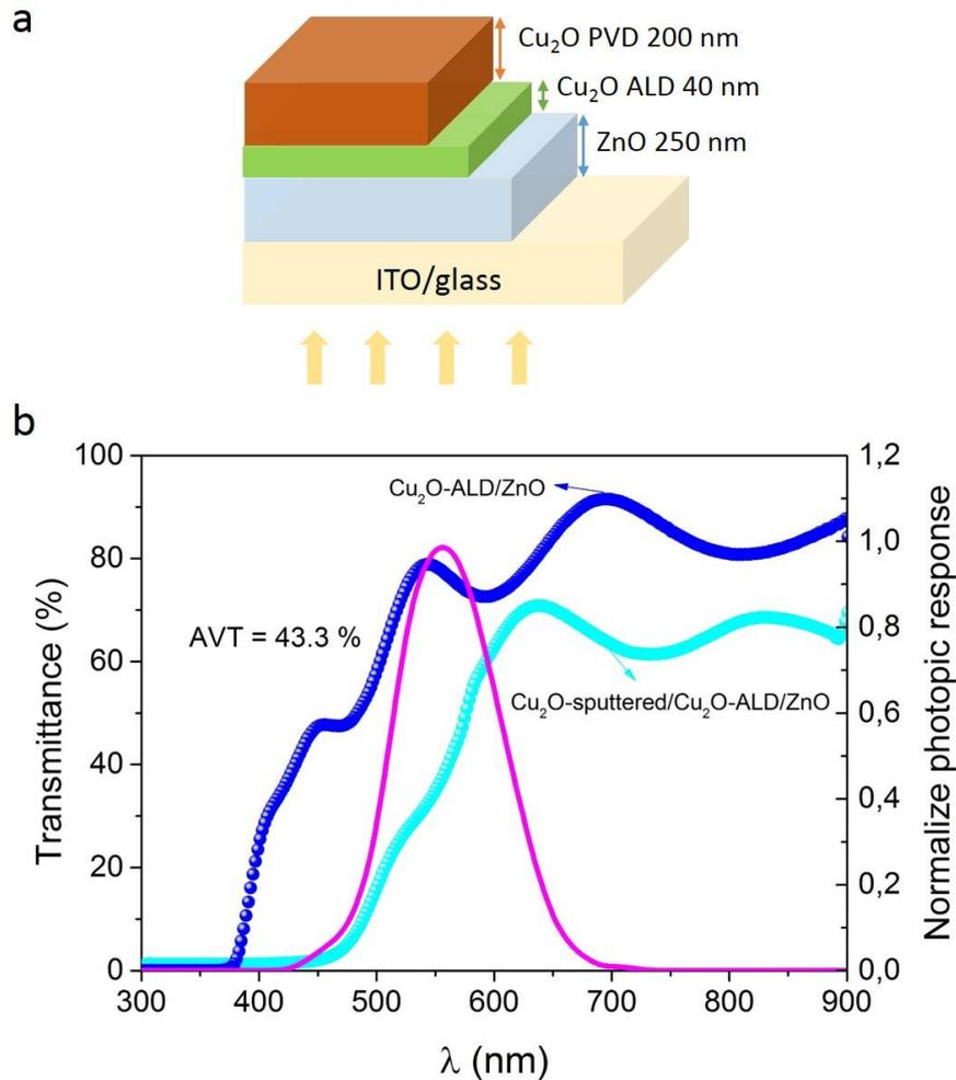
**Figure 5.12.** Schematic of the heterojunction with the addition of an uppermost Cu<sub>2</sub>O layer growth by sputtering (a). Transmittance of the Cu<sub>2</sub>O-ALD/ZnO (blue), Cu<sub>2</sub>O-sputtered/Cu<sub>2</sub>O-ALD/ZnO film (cyan) and the normalize photopic response of the human eye (violet) (b).
